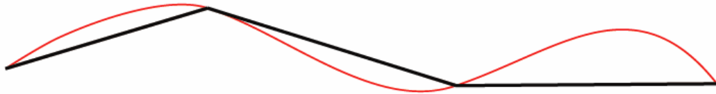
Figure 4.2: Spline Approximation. Red curve is the spline which has been roughly approximated by assuming just two values of 0 and 1 as for its parameter
