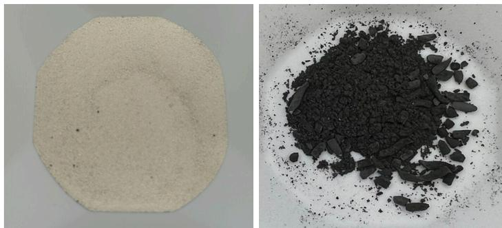
**Figure 9.** Photos of ZSM-5 before (left) and after (right) use in the reactor
