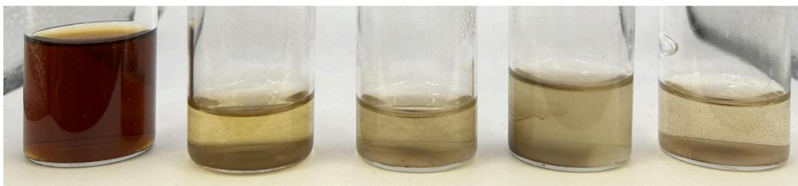
**Figure 5.** Pictures of HTL-AP samples before and after reacting at varying temperatures. From left to right: Unreacted HTL-AP, 380 °C, 400 °C, 420 °C, 440 °C.
