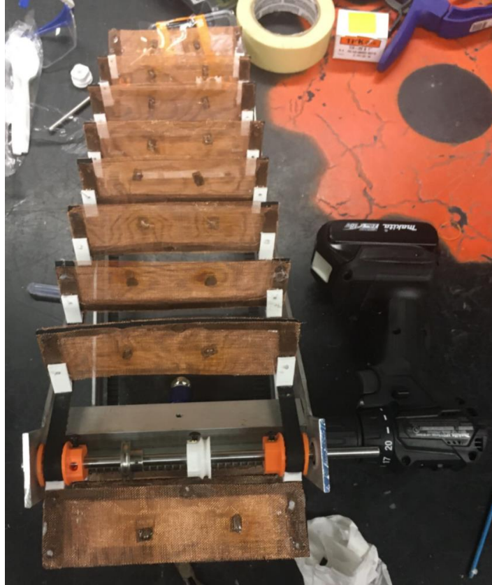
Figure 71. Testing Belt System Out of Box. The drill, on the right, was used to easily turn the axle, with a low torque rate and low speed, in order to simulate the motors being used in the final assembly.
