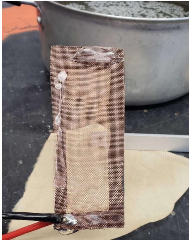
Figure 72. Test Paddle. This test paddle has slightly less interior surface area than the actual paddles on the assembly, as additional interior spacers were required to account for the heavier jumper wires used in this test.
