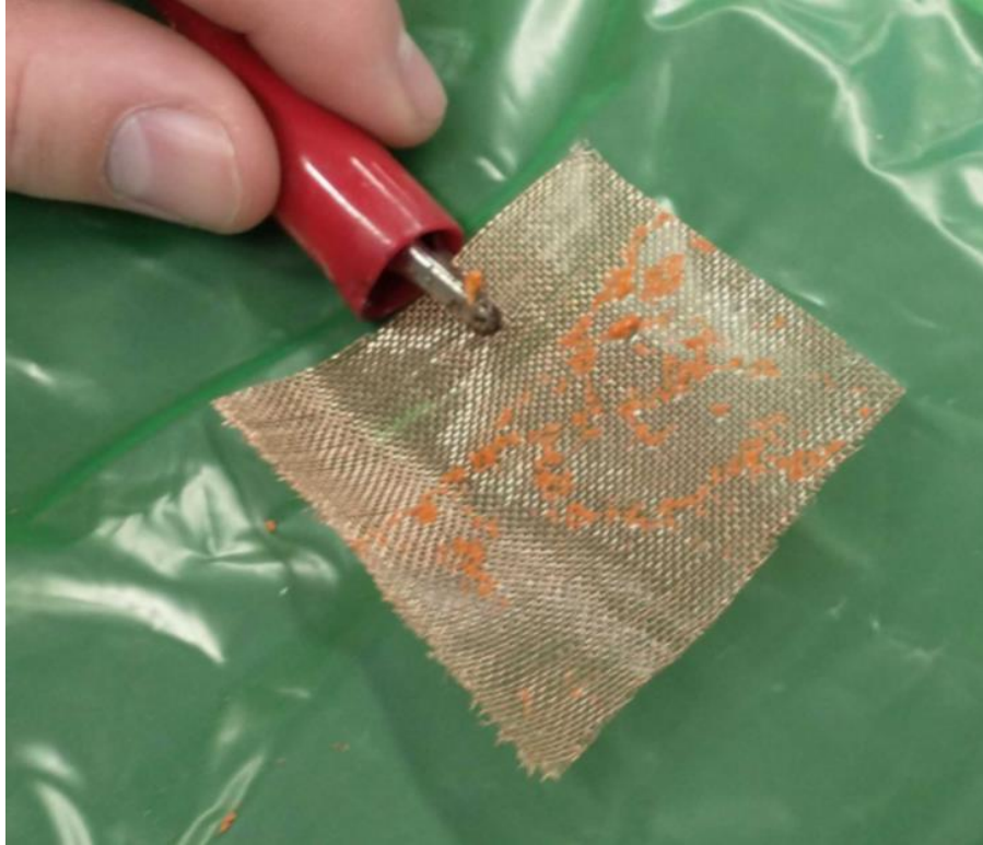
Figure 70. Testing Microplastic Electrostatic Charge. The orange plastic particles collected on electrically charged 0.5mm copper mesh.
