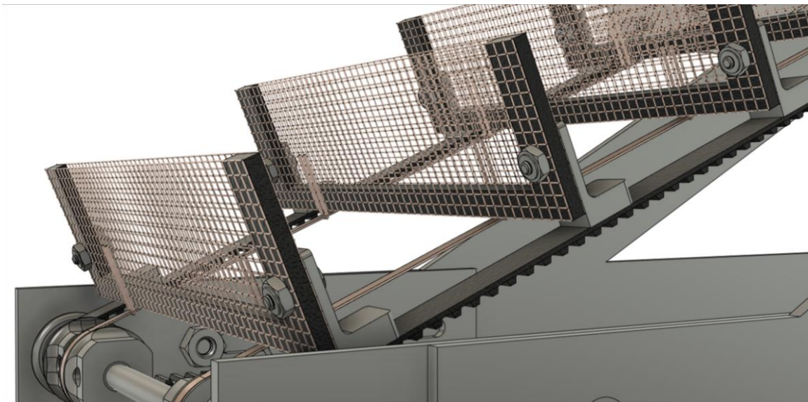
Figure 27. CAD Render of the Mesh Paddles and Electrostatic Rail
