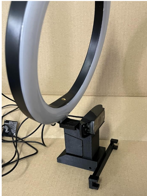
Figure 7.36: Full assembly of the RepRap camera fixture
