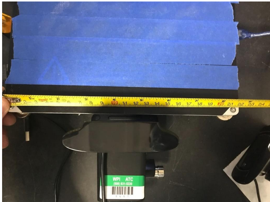
Figure 6.2: How the camera was centered relative to the print bed. The lens of the webcam was placed at 110 mm (half of the width of the print bed)
