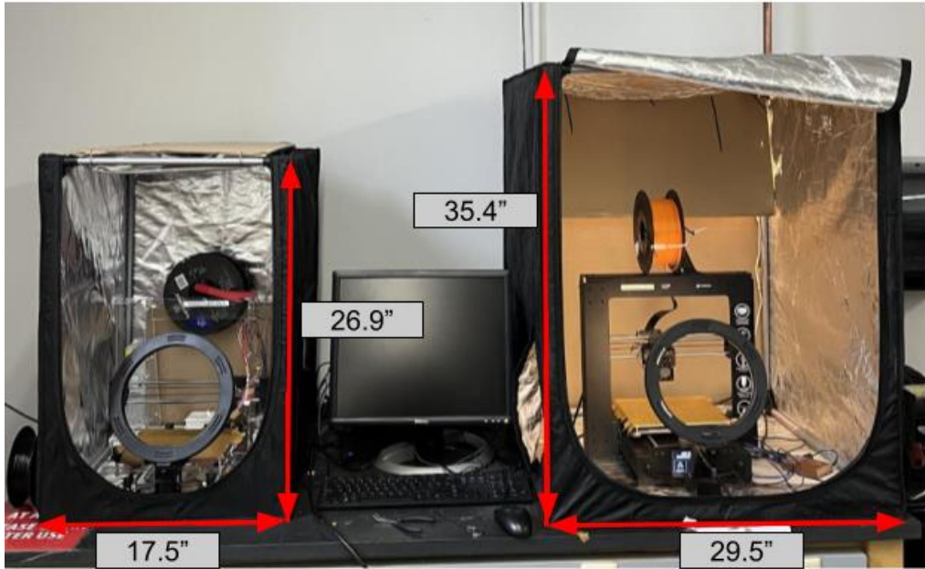
Figure 7.1: Enclosures with width and height dimensions. RepRap printer with small enclosure shown on the left. MonoPrice printer with the large enclosure shown on the right
