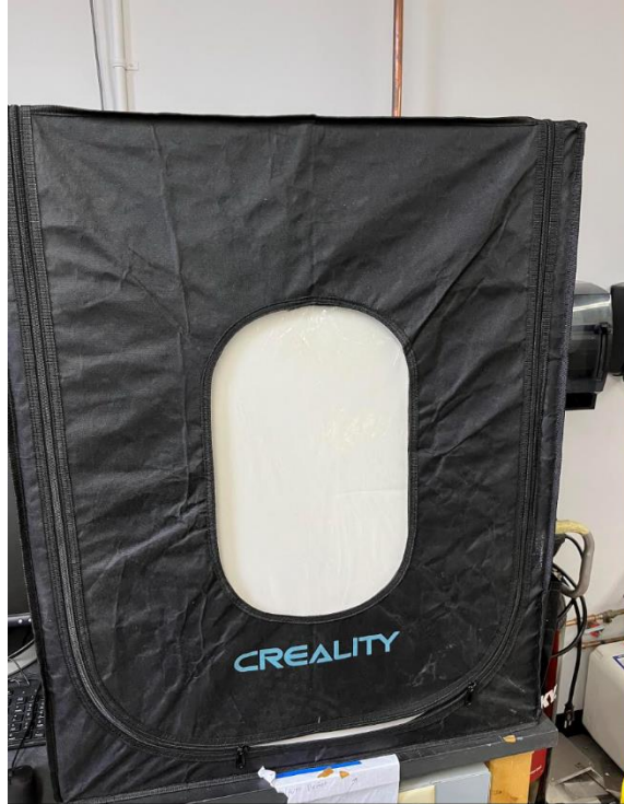
Figure 7.6: Large Monoprice enclosure closed with the poster board window barrier in place
