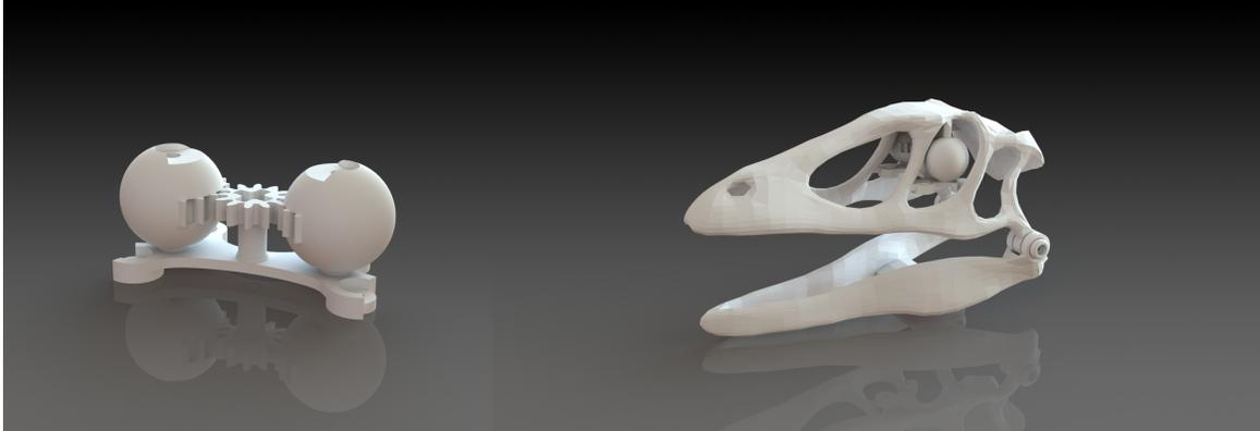
Figure 29: The eye assembly alone and mounted in the skull.
