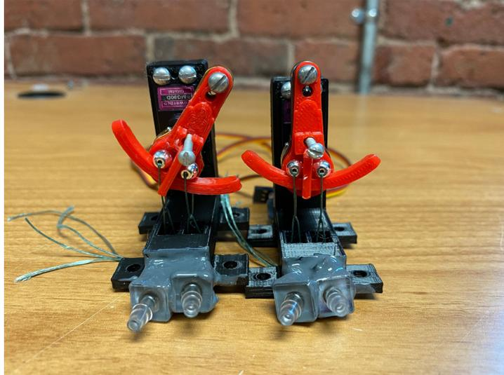
Figure 9: CRFC valves, left closed & right open (left) and both closed (right)
