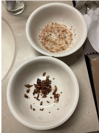
Figure 9: The result of separation of a pulverized mixture using a 35% saltwater solution. The above bowl contains what floated, and the bottom bowl contains what sank.
