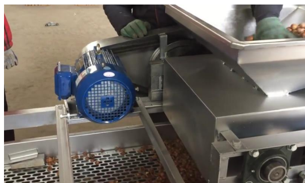
Figure 2: The Henan Ruiya sifting machine.
