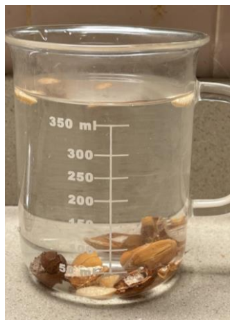
Figure 7: The argan shells sink in regular tap water while the argan kernels mostly float.
