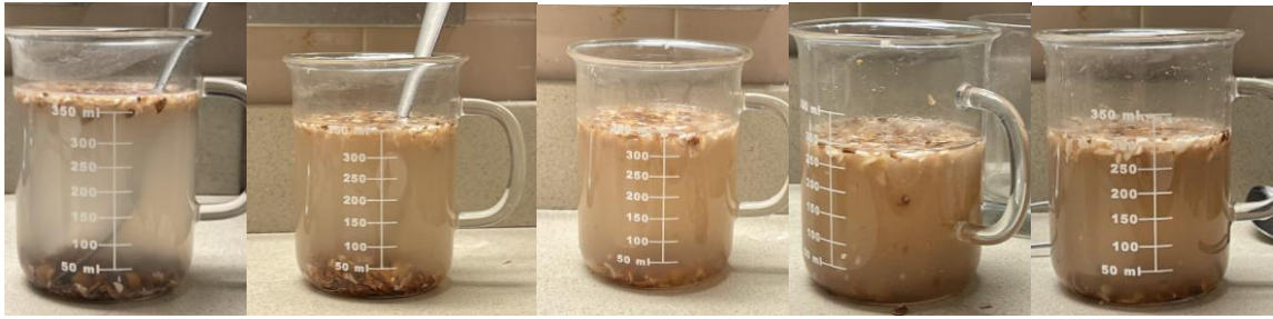
Figure 11: The progressive browning of the saltwater with each successive round of separation.
