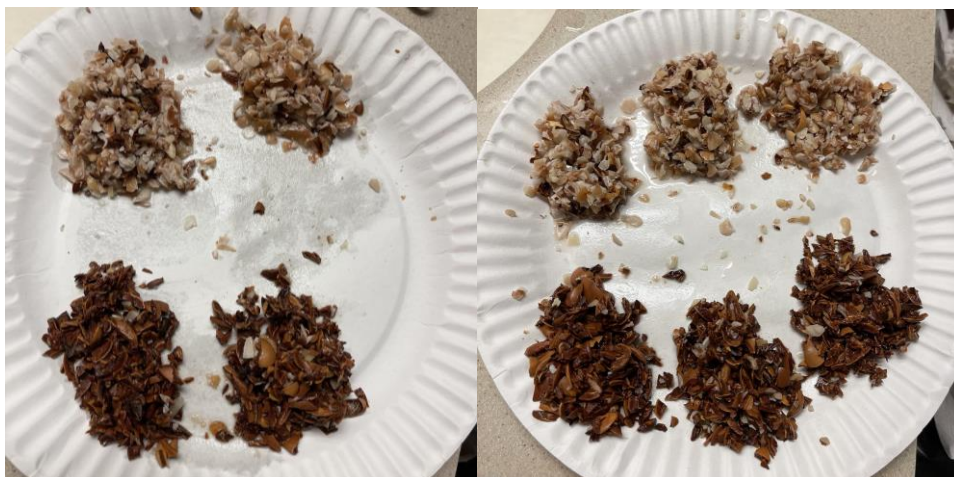
Figure 10: The separation results of each successive round of tests reusing water. The first test produced the leftmost two piles, the second two piles from the left, etc.
