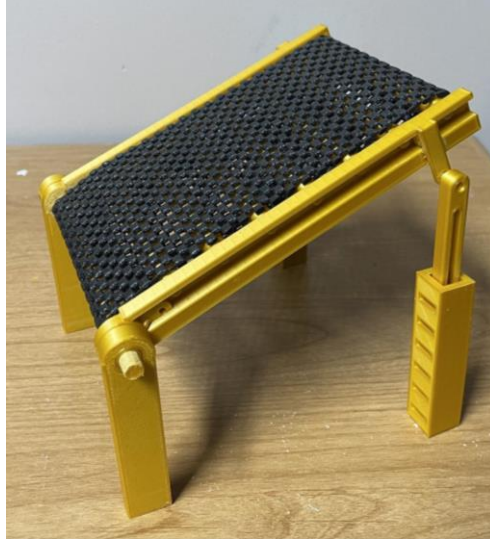
Figure 6: The fully built conveyor belt.
