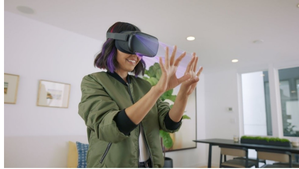
Figure 2.7: The Oculus optical finger tracking uses the headset's cameras to track the user's hands and fingers [8]
