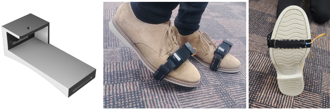
Figure 3.18: The SDP design (left), user with SDP (center), and force sensor location (right)
