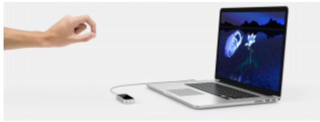
Figure 2.5: Leap Motion connected to a computer and tracking hand [22]
