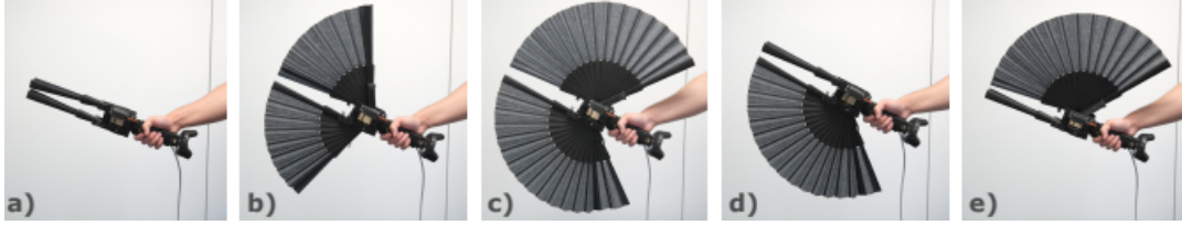
Figure 2.18: Different Output Configurations of the Drag:on VR controller [29]
