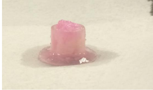
Figure 15: PVA Swelling out of a Scaffold PVA swelled during degradation to the point that it is extruding the hydrogel cell suspension.
