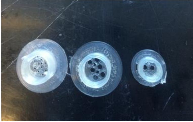
Figure 17: Different Threaded PLA Scaffold Designs
