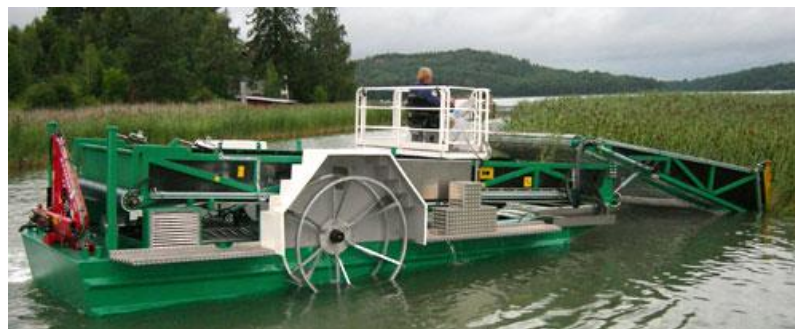
Figure 3: Aquatic Plant Harvester RS 2000 (RS Planering Ltd, 2008)
