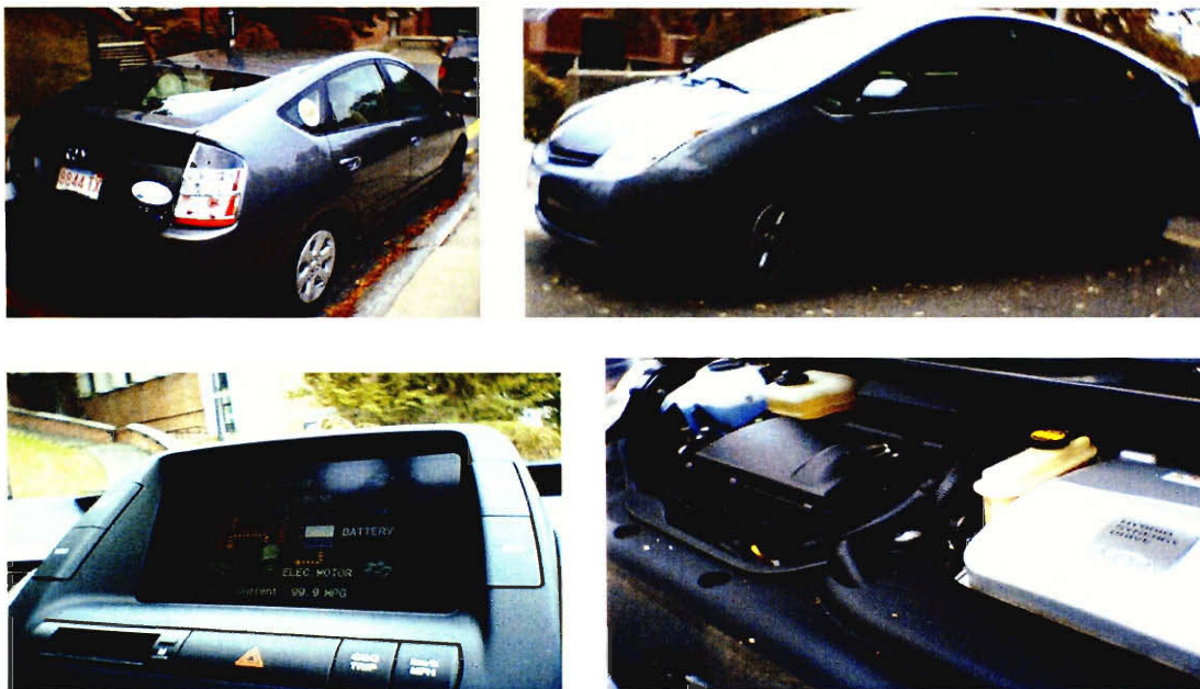
Figure 12: The pictures above are of the 2004 Toyota Prius model we tested. Rear offset photo (Top Left), side offset photo (Top Right), Multi-Informational Display (Bottom Left), under the hood: 1.5-Liter engine with Toyota's Hybrid Synergy Drive (Bottom Right). (Robert Dandekar)
