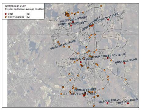
Figure 45 Signs in poor and below average condition
