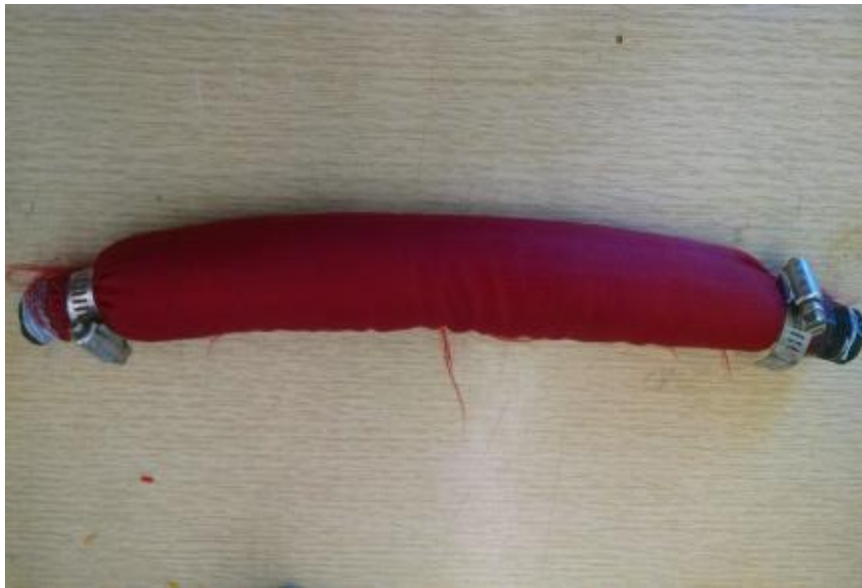
Figure 5: 1 st Generation HydroBone utilizing granulated EPDM rubber
