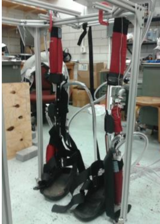
Figure 13: Variable Stiffness HydroBone Exoskeleton
