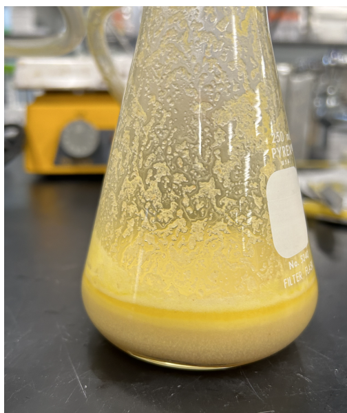
Figure 57: The oil froth that was suctioned out after the decanting period. Oil can be seen as well as fibers and a large amount of DPBS.
