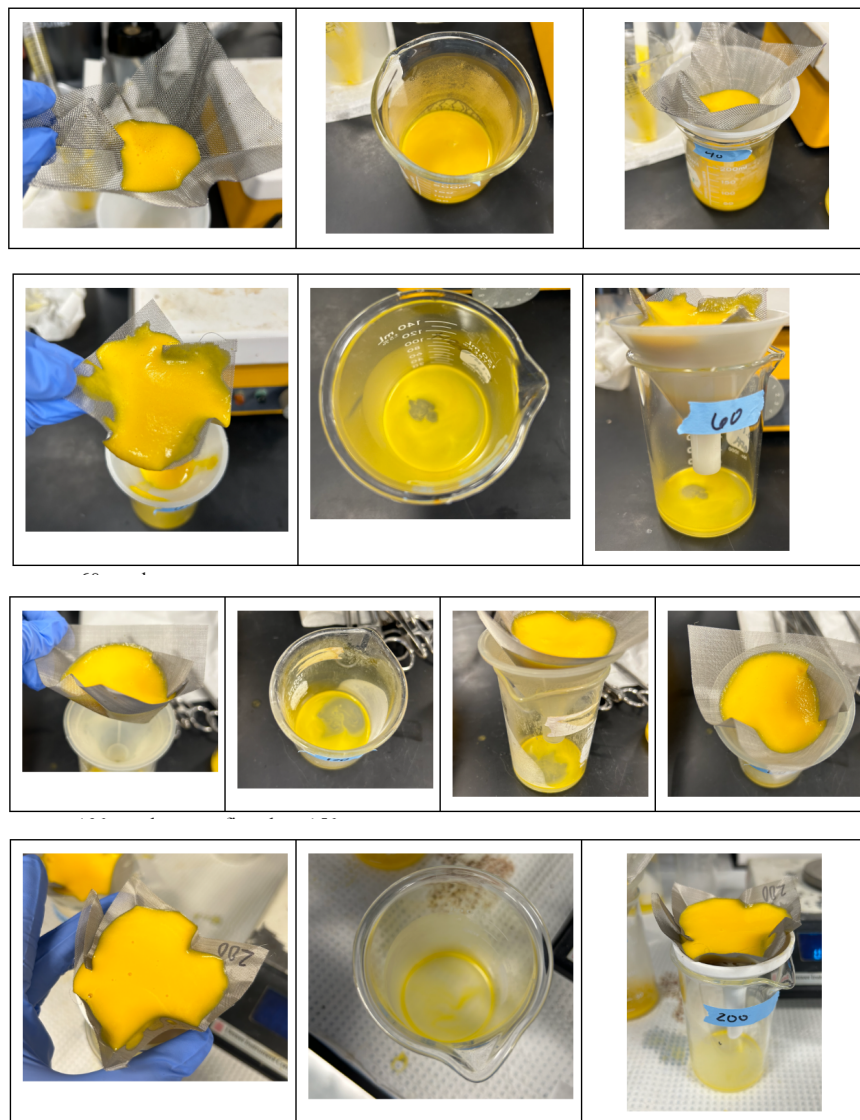
Figure 53: Mesh testing for gravity filtration results from top to bottom: the 40 mesh, 60 mesh, 120 mesh, and 200 mesh.
