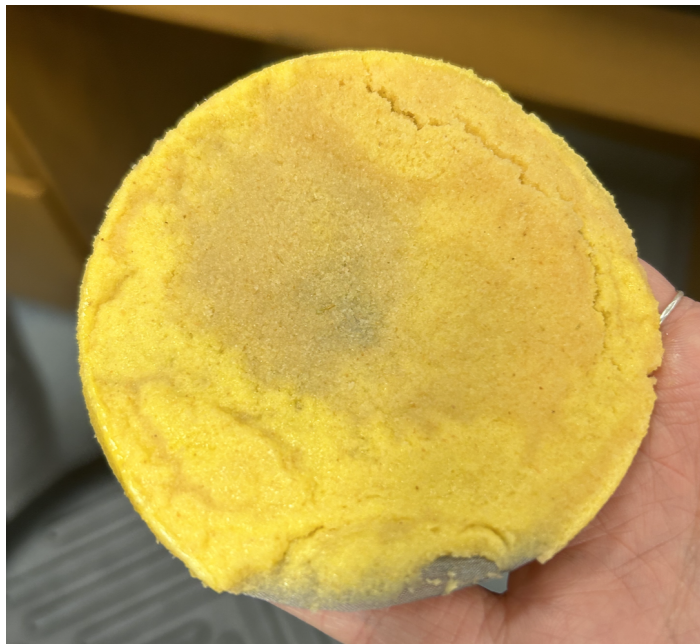
Figure 58: After suctioning out as much oil as possible and running the rest of the mixture through the set up most of the solids stayed on top and were mostly dry of any DPBS. However some oil was still trapped on top as well as some areas were still wet with DPBS.
