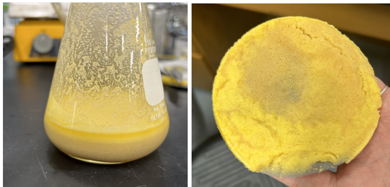
Figure 5: Liquid waste removed on the left and solid product above the mesh filter on the right.
