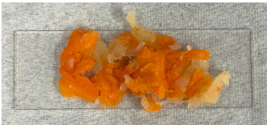
Figure 37: Mashed carrot used to replicate lipoaspirate. Has a similar texture to lipoaspirate, it has fibers, water within the cells so when broken it should release the liquid and leave behind the fibers and ECM.
