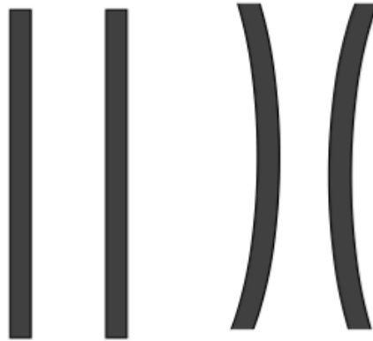
Figure 21. (Left) Two Pane IGU with No Deformation. (Right) Two Pane IGU with Deformation Causing Concave Shape 3
