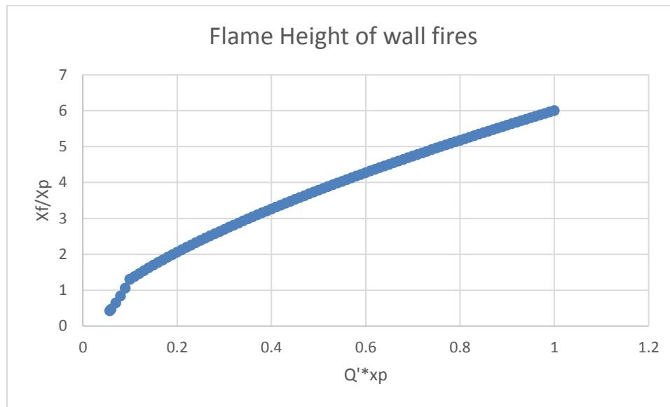
Figure 48: Flame heights of wall fires
