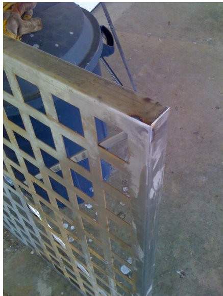
Figure 4- Welded corners ground smooth
