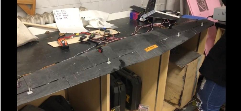
**Figure 63: Ailerons and flaps control surfaces**
