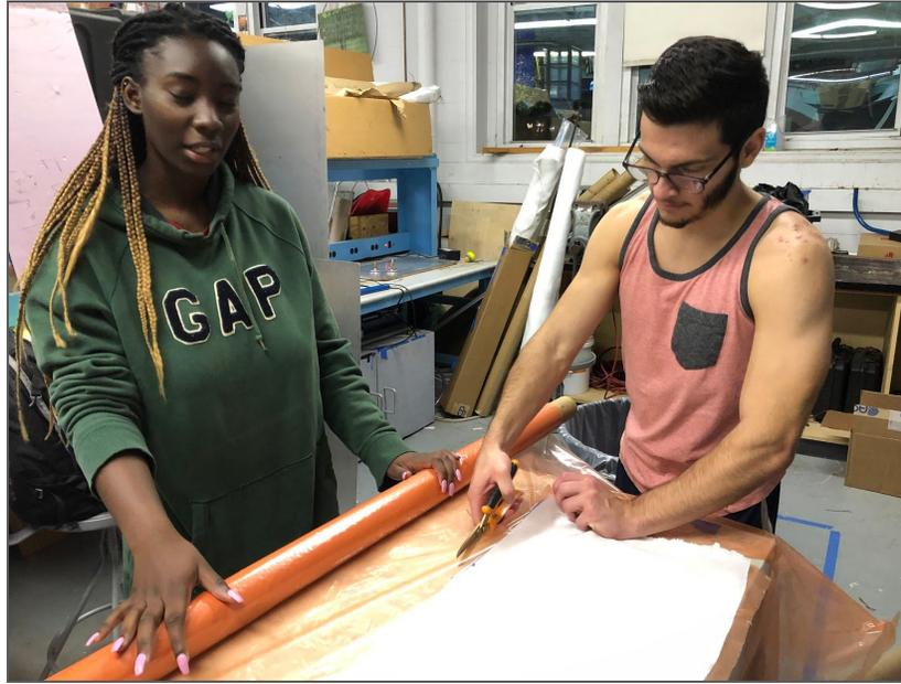
**Figure 58: Cutting Breather and Wadding**
