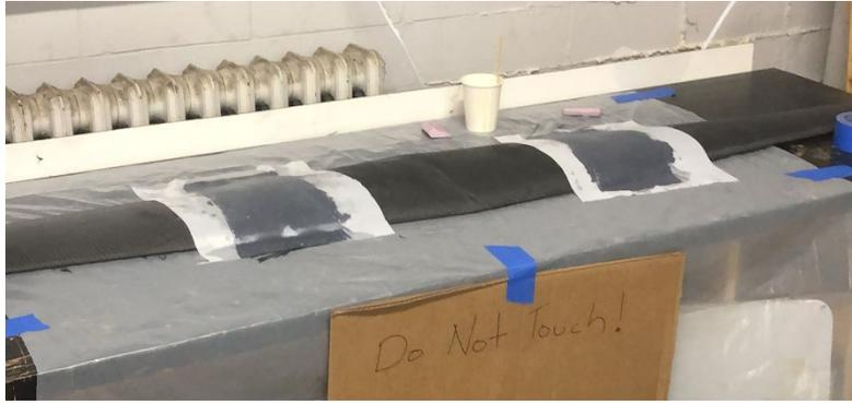
**Figure 61: Wing Assembly Lay-up**
