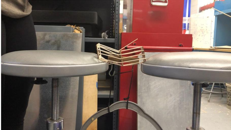
**Figure 81: Fuselage Failure During Loading Test**
