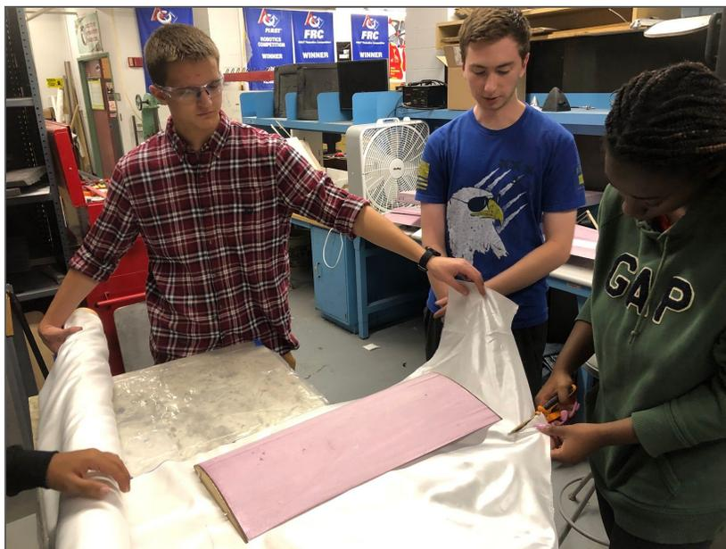
**Figure 57: Cutting Peel-Ply**
