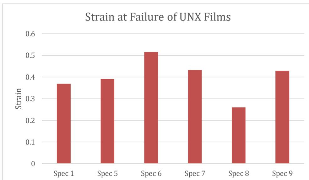
Figure 28. UNX Strain at Failure
