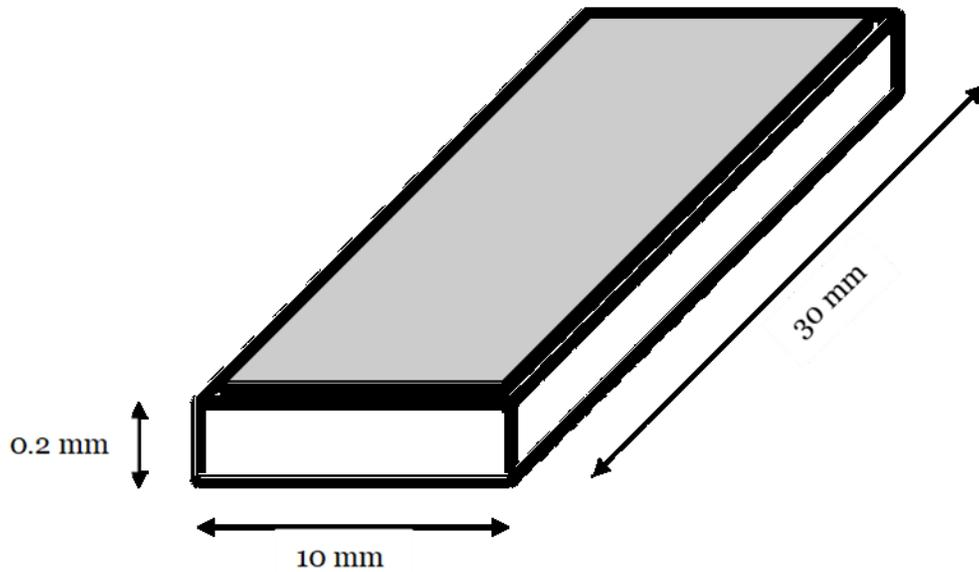
*Figure 20. Schematic of Film with Sponge*
