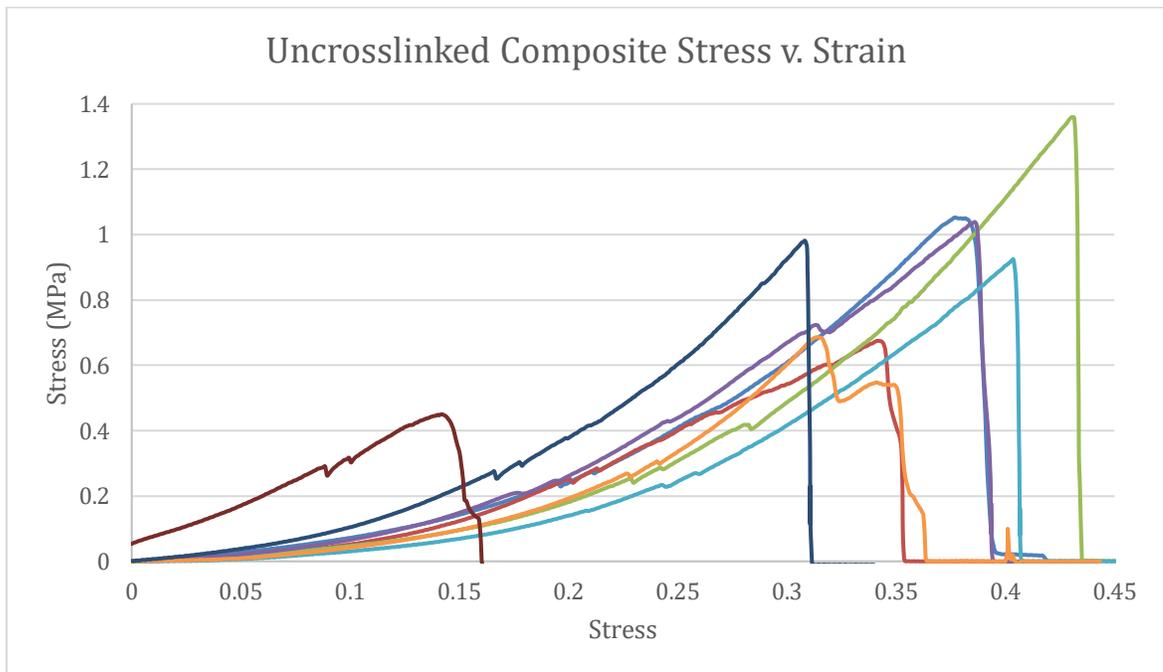
Figure 32. UNX Composites Stress vs. Strain
