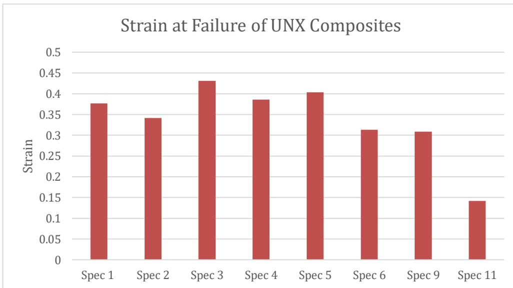
Figure 34. UNX Composite Strain at Failure
