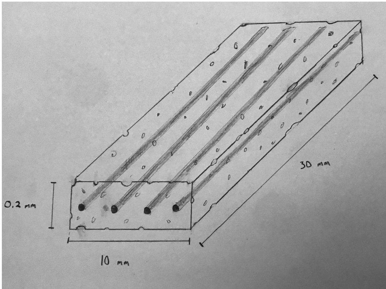
*Figure 21. Schematic of Sponge with Threads*
