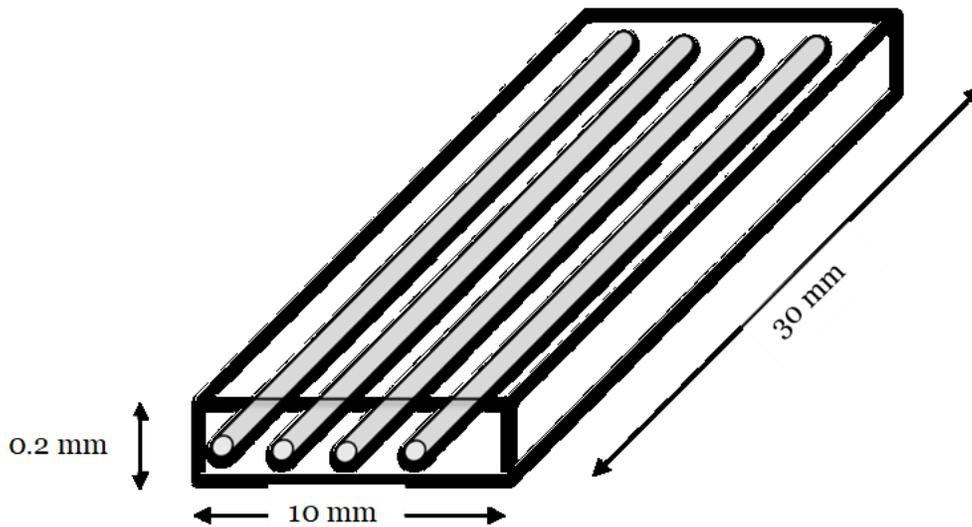
*Figure 19. Schematic of Film with Threads*
