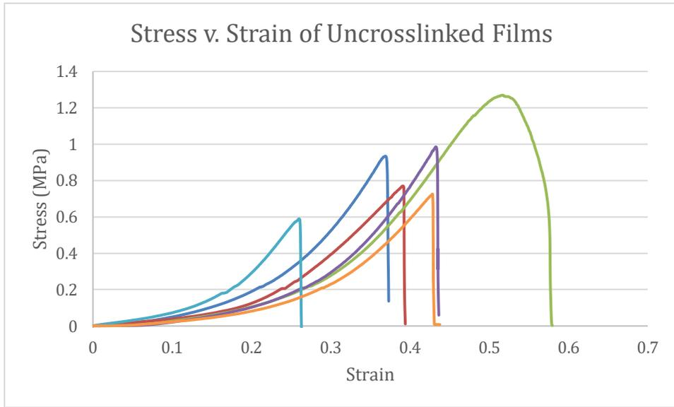
Figure 26. UNX Films Stress vs. Strain
