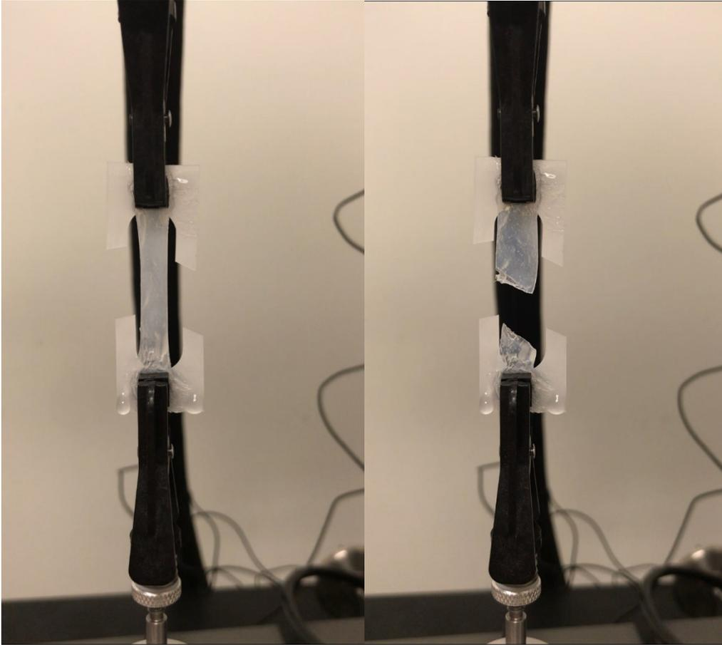
*Figure 25. Instron Set up for Tensile Testing*
