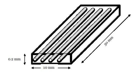
Figure 19. Schematic of Film with Threads
