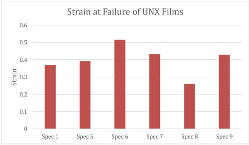
Figure 28. UNX Strain at Failure
