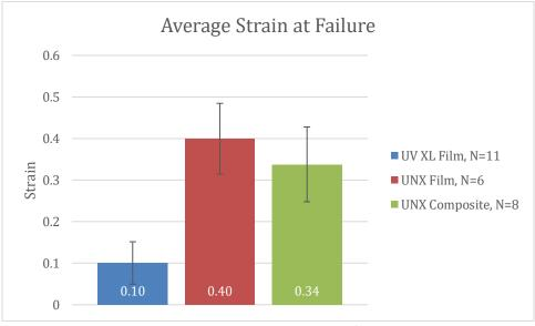
Figure 37. Average Strain at Failure
