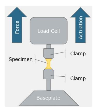
Figure 24. Instron Setup Schematic
