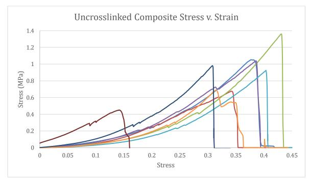
Figure 32. UNX Composites Stress vs. Strain
