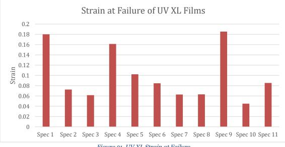
Figure 31. UV XL Strain at Failure
