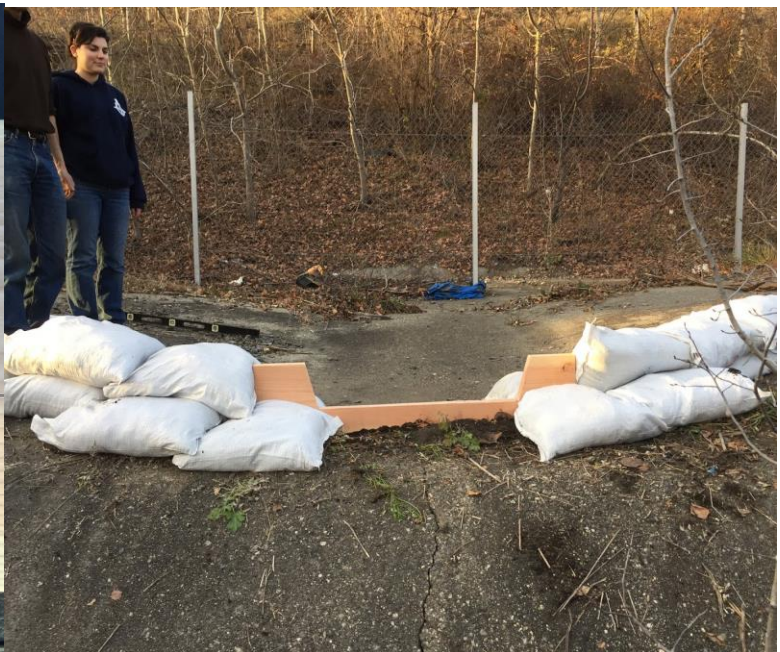
FIGURE 11: SETUP OF WEIR WITH SANDBAGS
