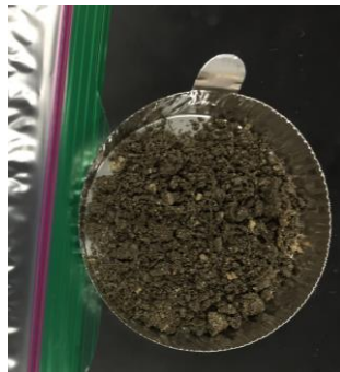
FIGURE 68: PLACEMENT OF SOIL SAMPLE ON PAN
