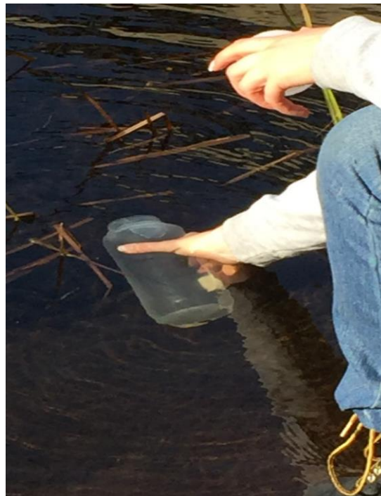
FIGURE 9: SUBMERGED SAMPLE BOTTLE
