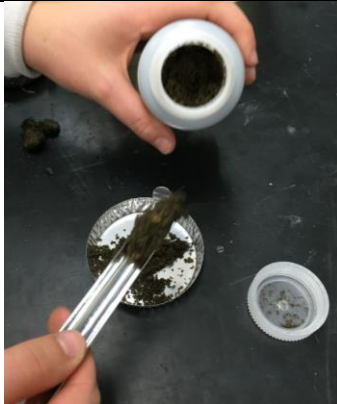
FIGURE 68: PLACEMENT OF SOIL SAMPLE ON PAN
