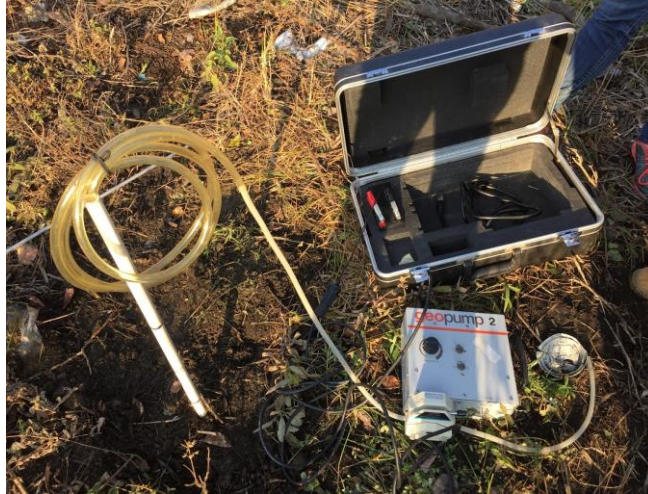
Figure 6: Groundwater Sampling Device with Pump
