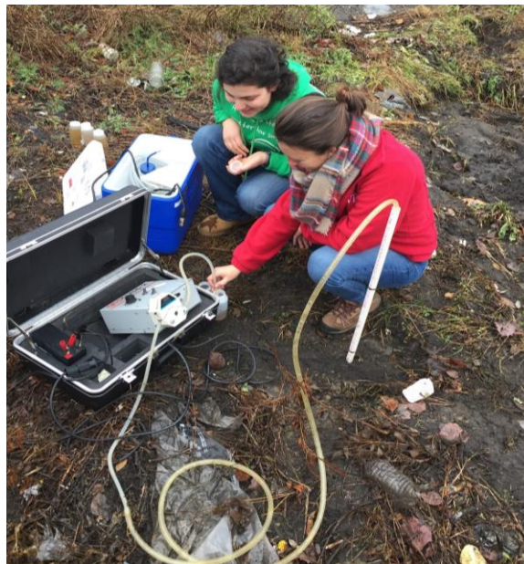
FIGURE 15: COLLECTION OF GROUNDWATER SAMPLES WITH GEOPUMP
