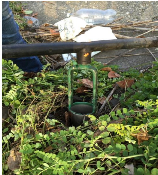
Figure 7: Taking Core for sample S2
