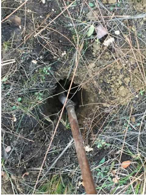
Figure 2: Coring device to dig hole
