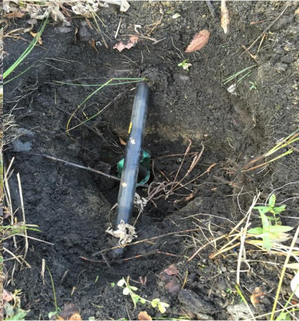
Figure 3: Removing Lower Soil with Coring Device
