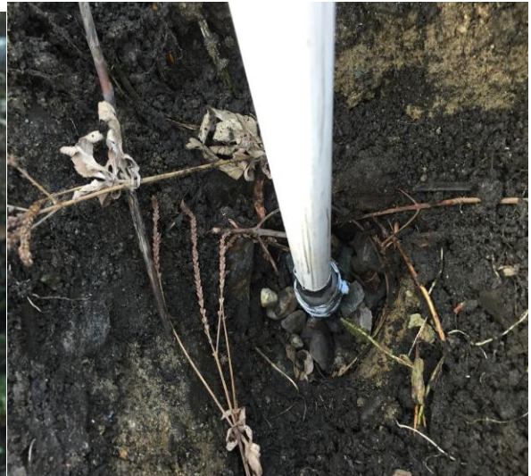
Figure 5: Groundwater Device Surrounded by Small Stones
