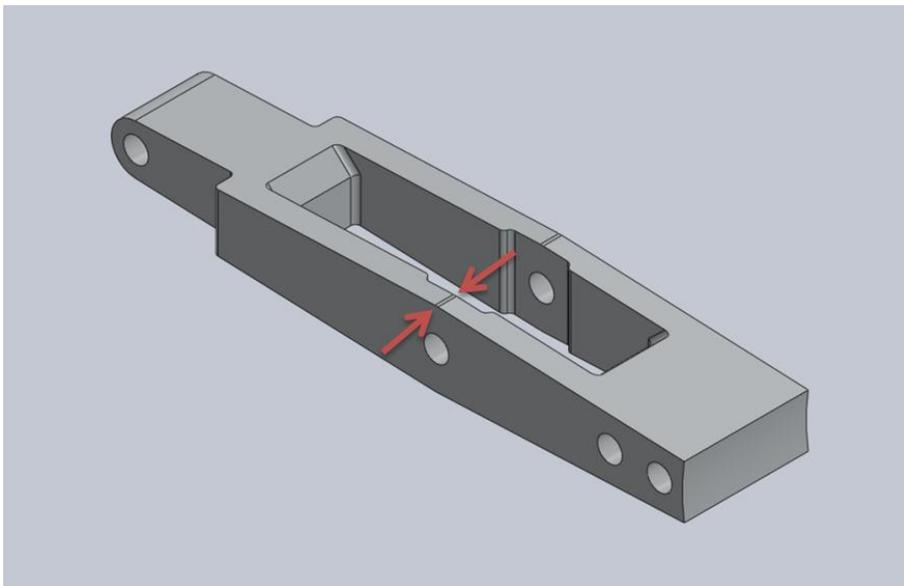
**Figure 19: Point of Highest Stress in the Lower Link**
