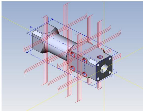
**Figure 40: Esprit generated 4-axis tool paths**
