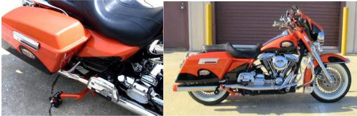
**Figure 9: Motorcycle outfitted with LegUp extended at rest (Left) retracted at rest (Right)**
