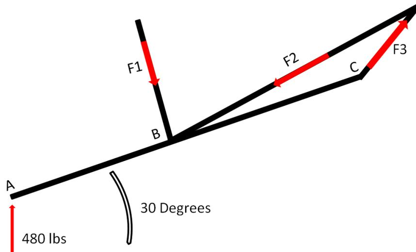
**Figure 20: Free Body Diagram of the Linkage**
