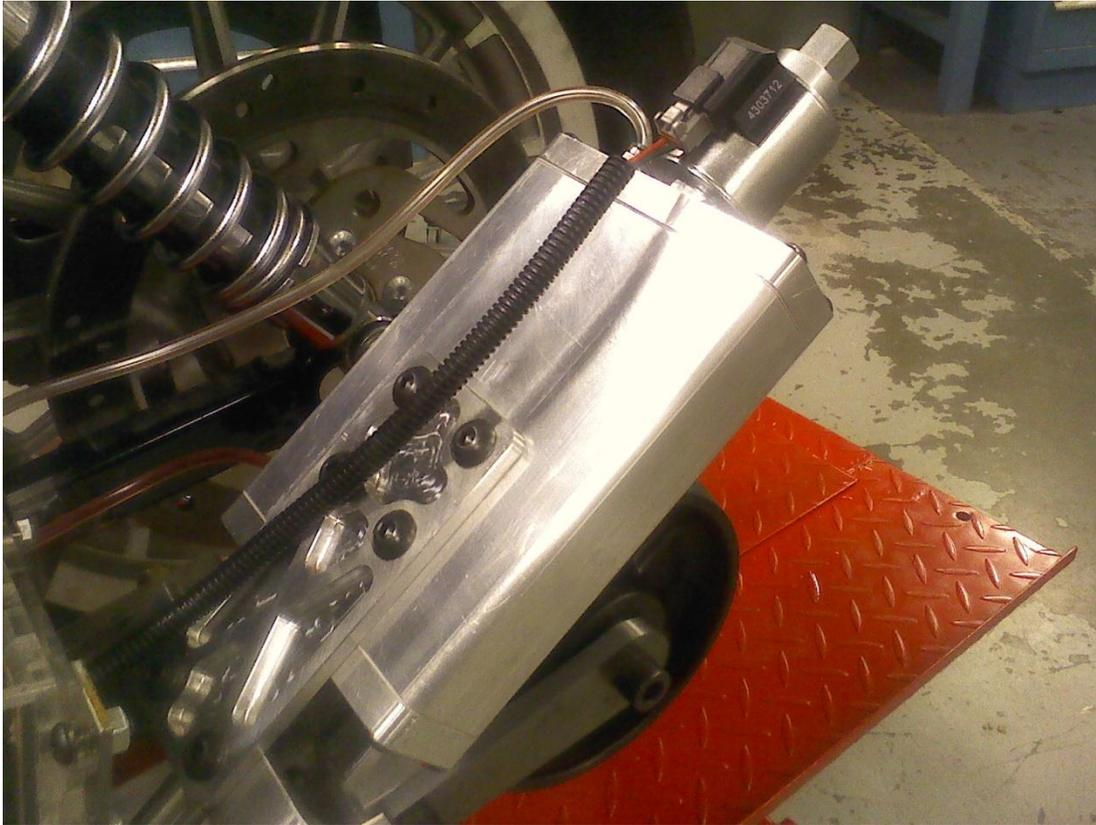
Figure 28: Installed Secondary Cylinder
