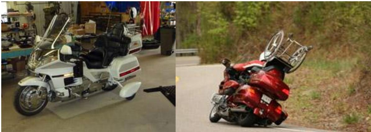
**Figure 8: Motorcycle outfitted with Retractable Trike extended at rest (Left) in motion (Right)**
