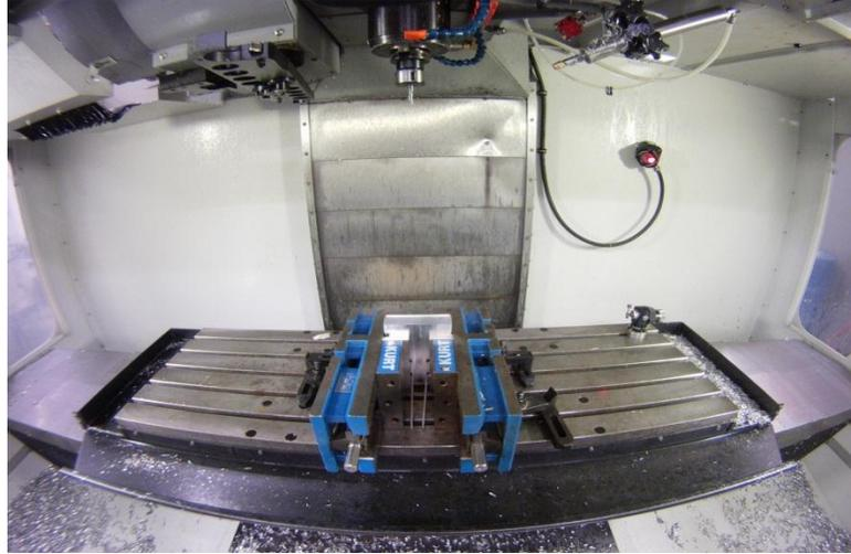
**Figure 39: Secondary Cylinder Body before drilling and reaming**
