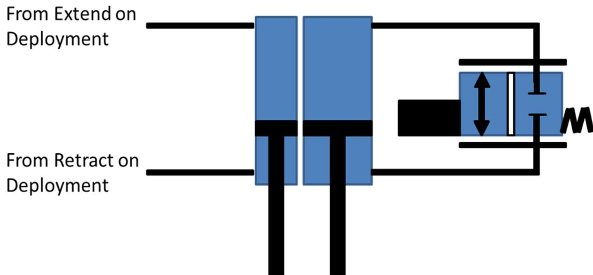
Figure 25: Secondary Cylinder Schematic
