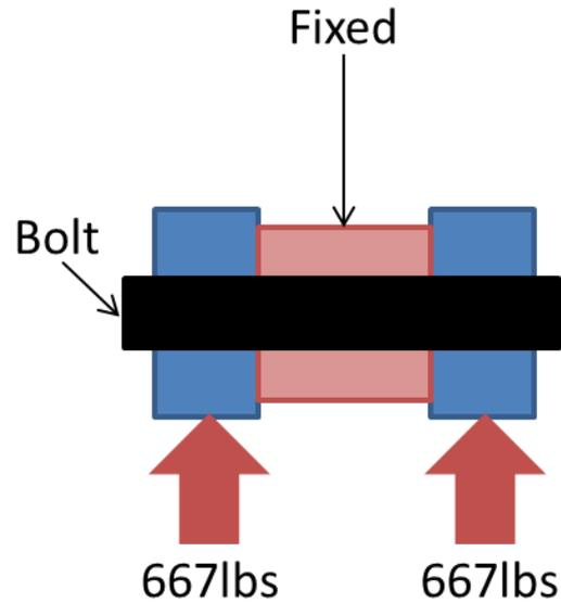
Figure 21: Diagram for pivot bolt in double shear
