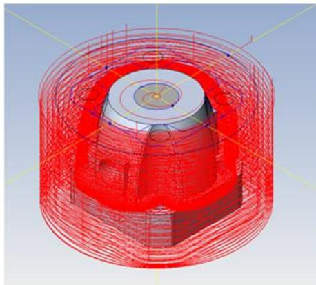
**Figure 42: Tool Path for Surface finishing**
