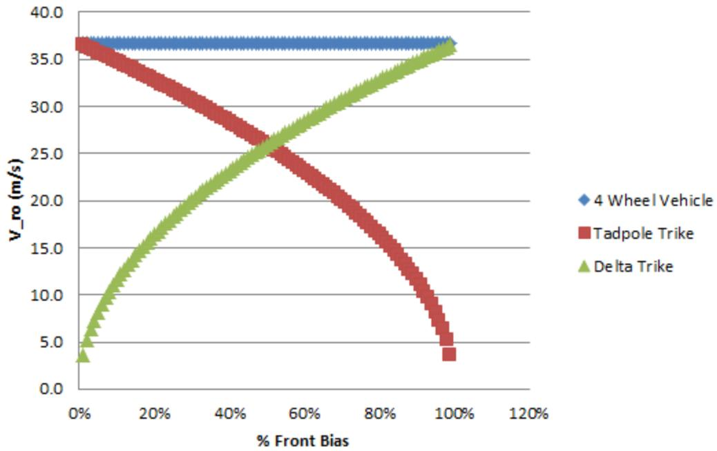
Figure 12: Rollover stability to Lateral Acceleration
