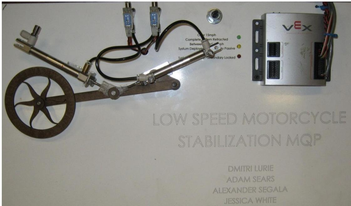
**Figure 30: Proof of Concept Model Using VEX Components**
