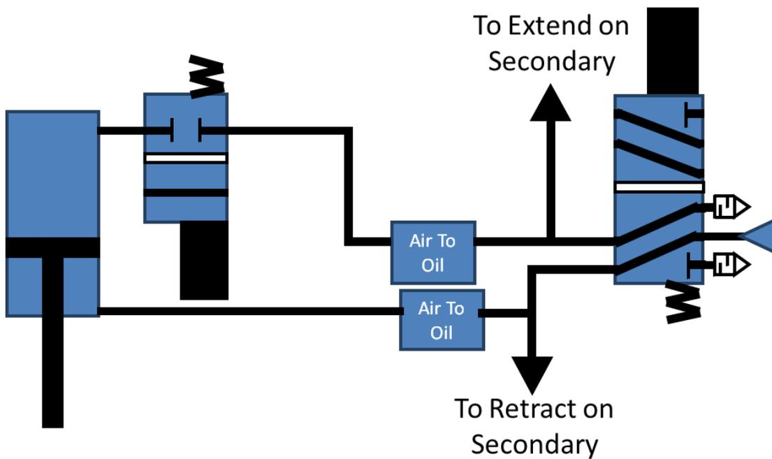
Figure 24: Deployment Cylinder Schematic
