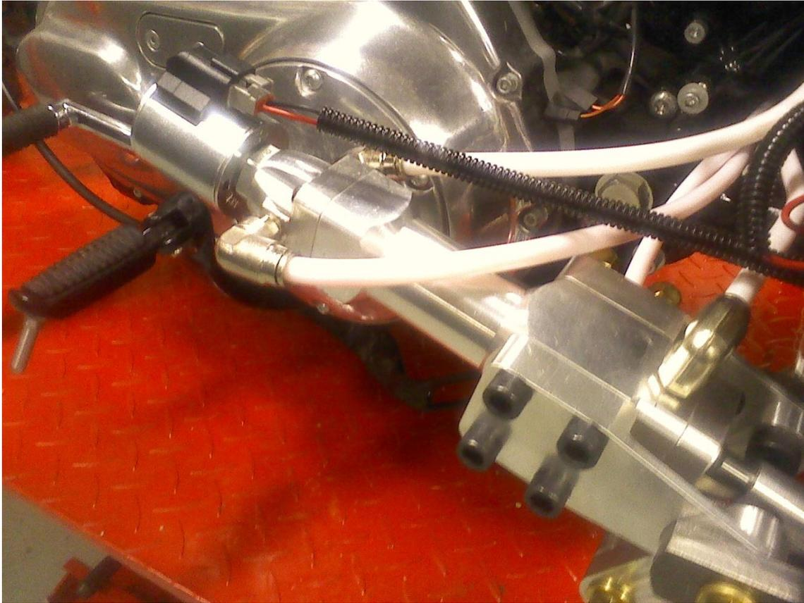
Figure 27: Installed Deployment Cylinder
