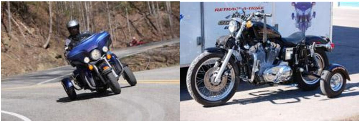
**Figure 7: Ghost Wheels Unlocked at Speed (Left) Locked in Stationary Position (Right)**
