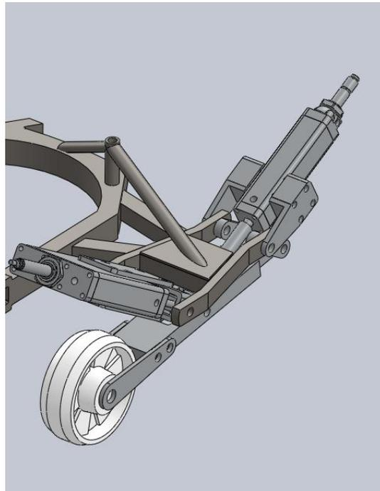
**Figure 38: Final Frame Model with Linkage Attached**
