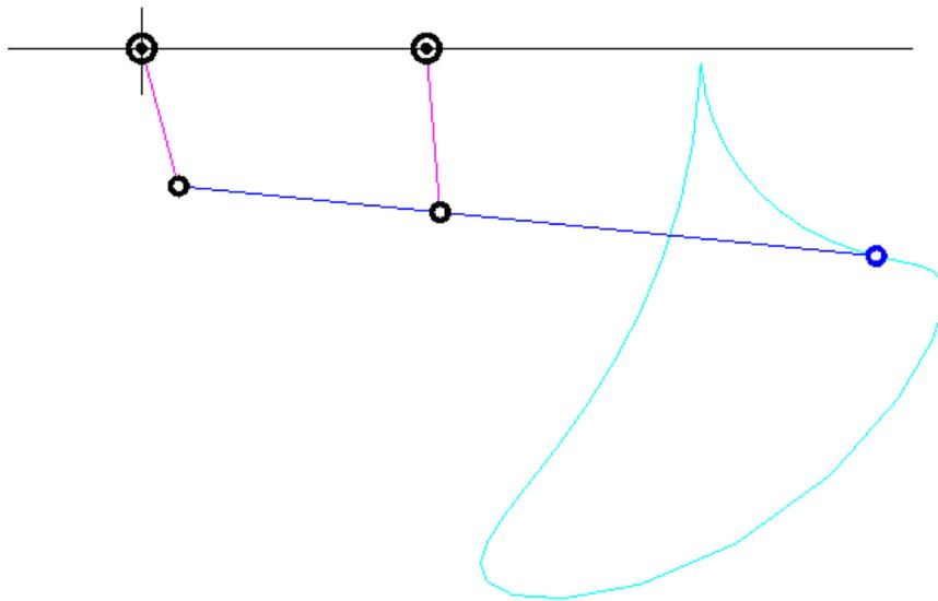
**Figure 17: Coupler Curve of Expanding Trailing Arm**
