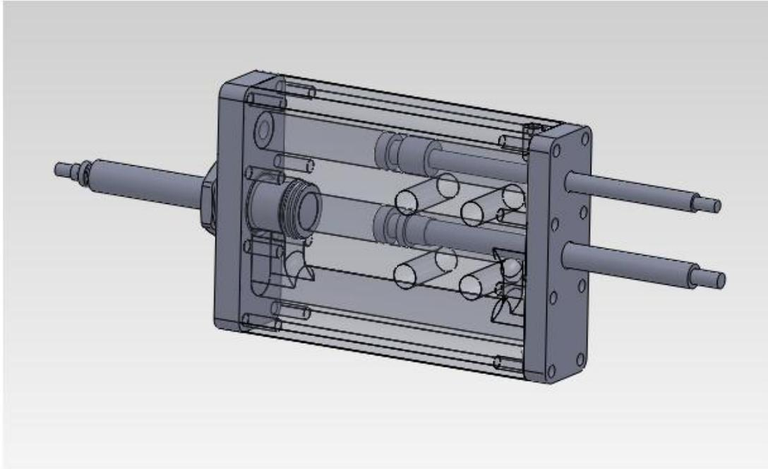
**Figure 29: Internal Configuration of Secondary Cylinder**
