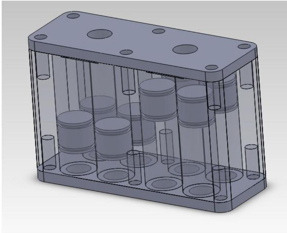
**Figure 26: Solid Model of Air to Hydraulic Converter**
