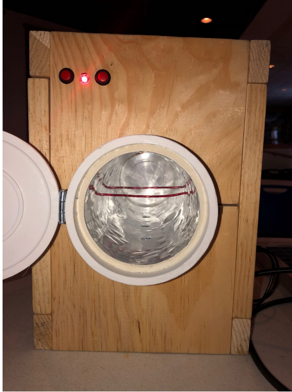
Figure 19: Open Sanitation Chamber
