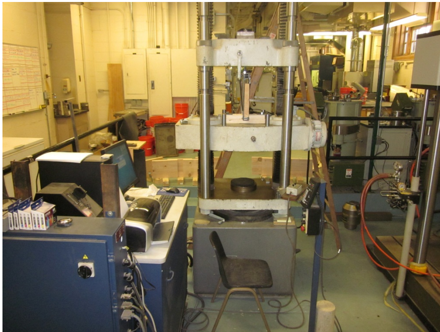
Figure 121: Tinius Olsen Universal Testing Machine
