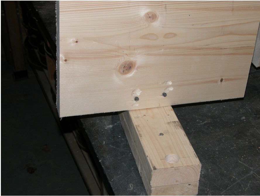
Figure 117: Toenail Connection Specimen
