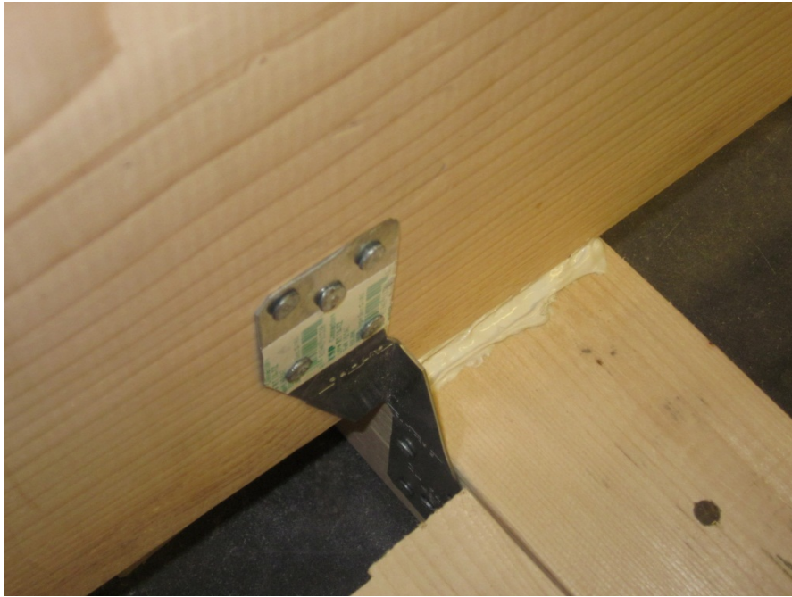
Figure 120: Liquid Nail and Hurricane Strap Connection Specimen
