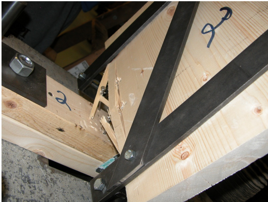
Figure 123: Deformed Toenail Connection Specimen
