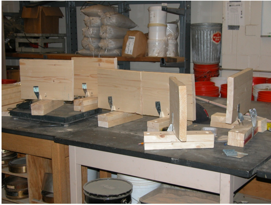
Figure 118: Toenail and Hurricane Strap Connection Specimens
