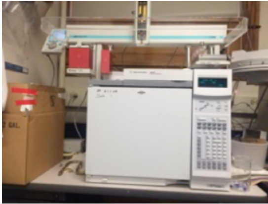
Figure B.5 GC-SPME-FID instrument
