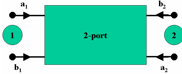
Figure 2.1. S -parameter representation of a 2-port system
