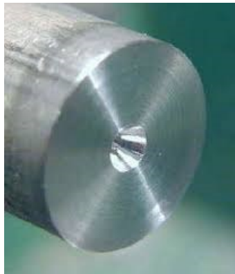
Figure 4. Tail-Stock center hole
