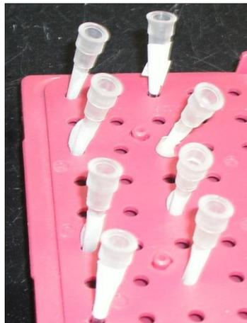
*Figure 5-1: Nylon Mesh configured into a conical shape*
