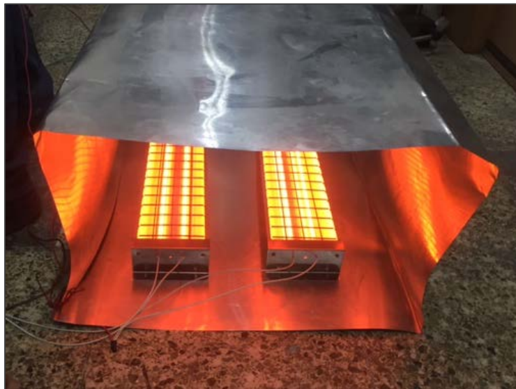
Figure 8: Heat containment box within IR tubes 10 cm apart
