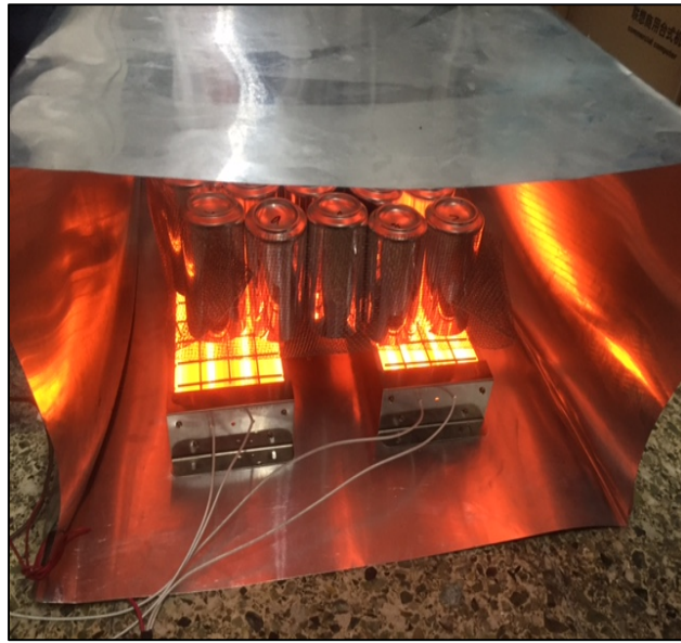
Figure 1: Heat containment box within IR Tube 10cm Apart
