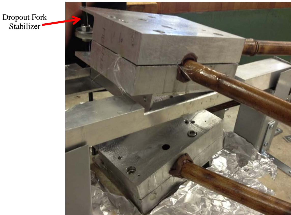
Figure 21: Dropout Mold Set Up
