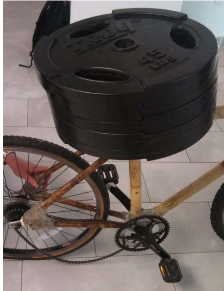
Figure 24: Static Loading Test
