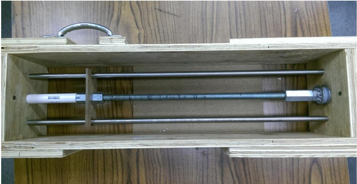
**Figure 3** lead screw type of drive system
