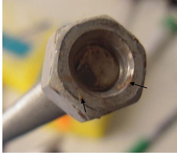
Figure 60: Epidermal layer residue (black arrows) on hex bolt.
