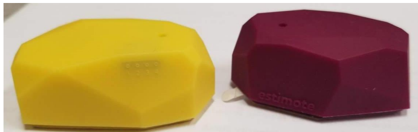
Figure 2.2: Two iBeacons developed by Estimote utilizing BLE Technology to Transmit Information that can be Detected by BLE Compatible Devices
