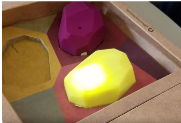
Figure 3.5: Estimote Beacon Producing Light to Notify User that the Beacon is Being Reconfigured by Owner
