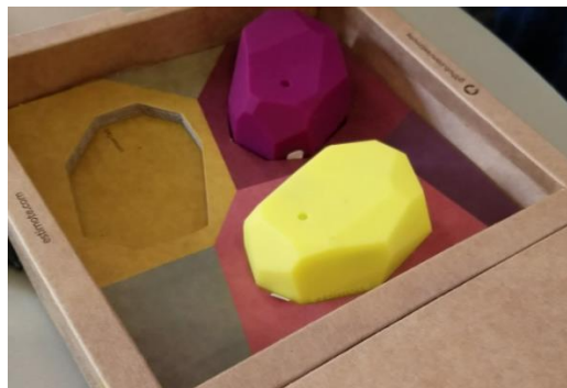
Figure 1: Estimote Location Beacons using BLE for promimity broadcasting for smart devices
