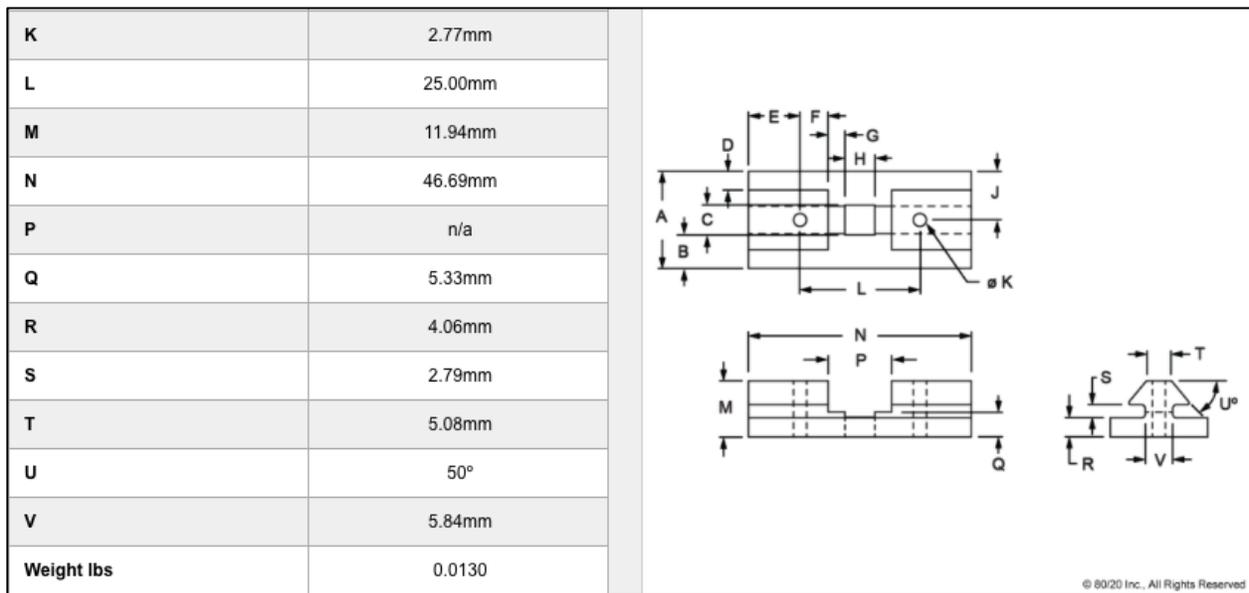
Figure 8: Critical Slider Geometry
