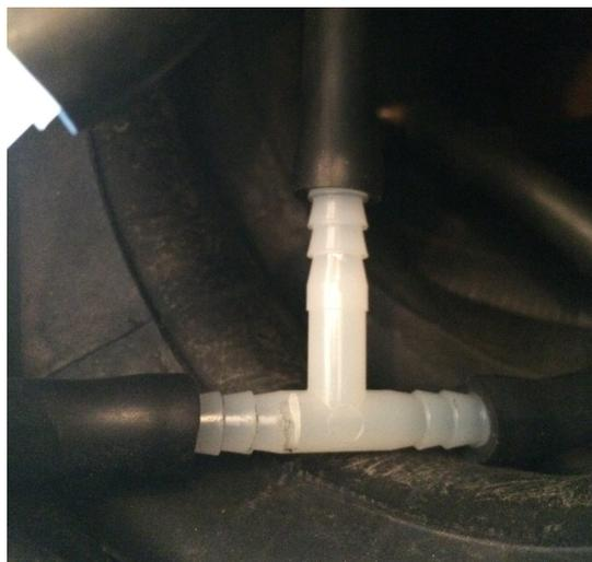
**Figure 16: T-Joint connected to vacuum hosing**
