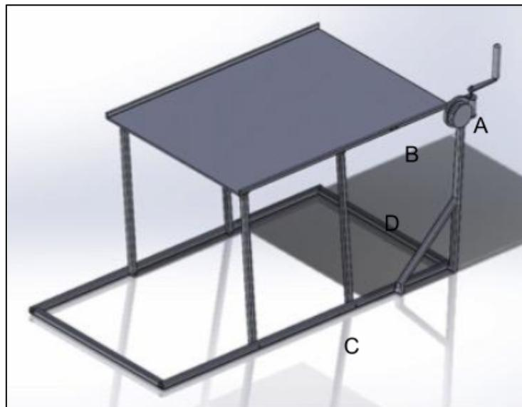
Figure 2: 4 Bar Winch Lift
