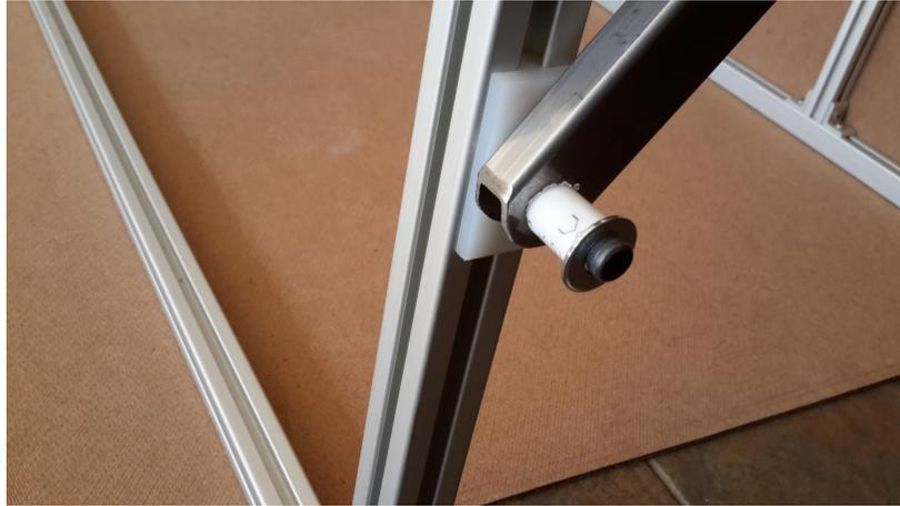
**Figure 13: Slider Assembly**
