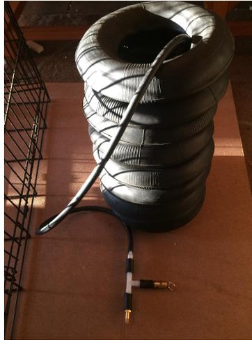
**Figure 18: Tire Stack Air Bladder**
