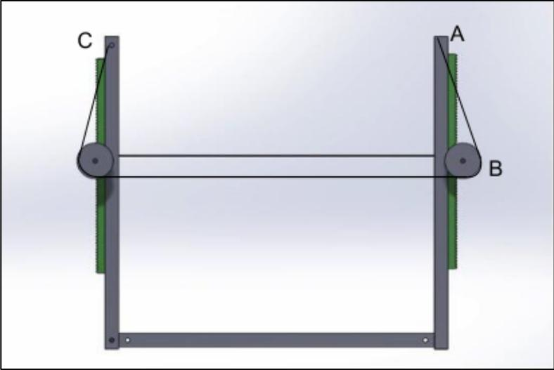
Figure 4: Rack and Pinion Concept
