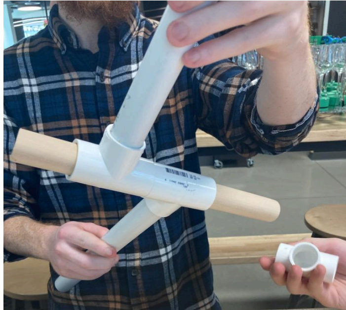
Fig. 30 - Wooden Dowel for PVC Rotation
