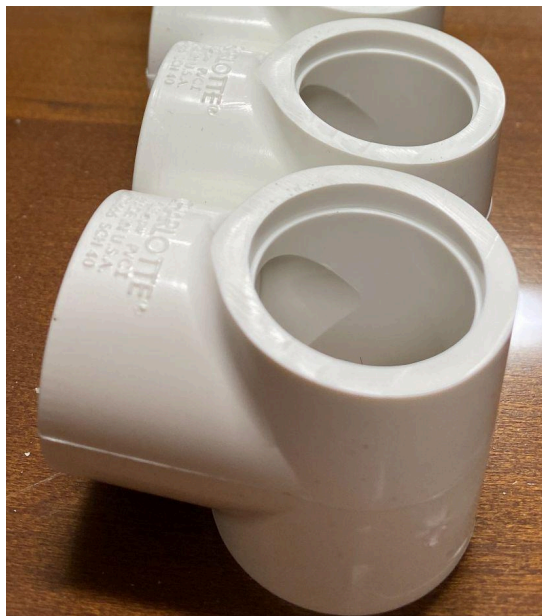
Fig. 28 - Cut \frac{3}{4} inch PVC T
