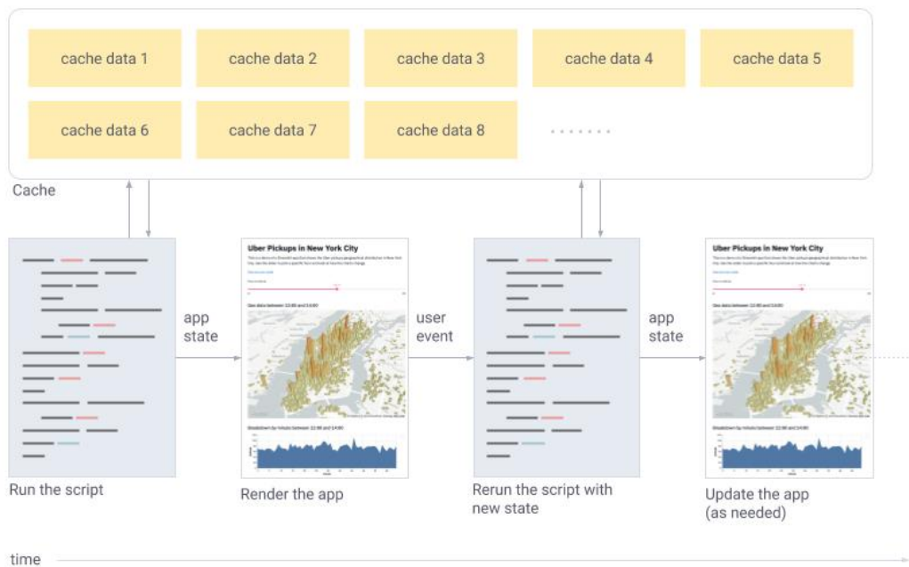
Figure 6 - Streamlit Web App Flow (Streamlit Inc., n.d.)
