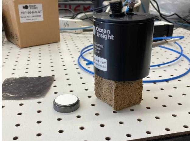
*Figure 21. Zoomed Experimental Setup for Measuring Reflectivity of the ECM-n Sample.
