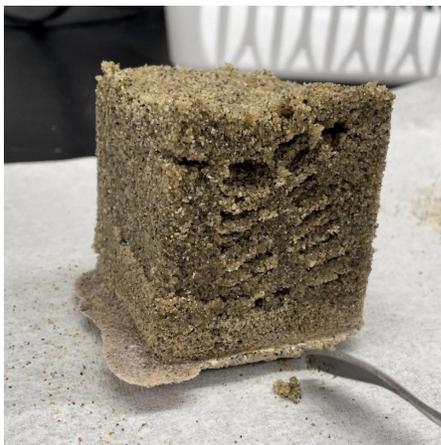
*Figure 18. Partially Cured 2" Cube ECM-n Sample Flipped Upside Down.*
