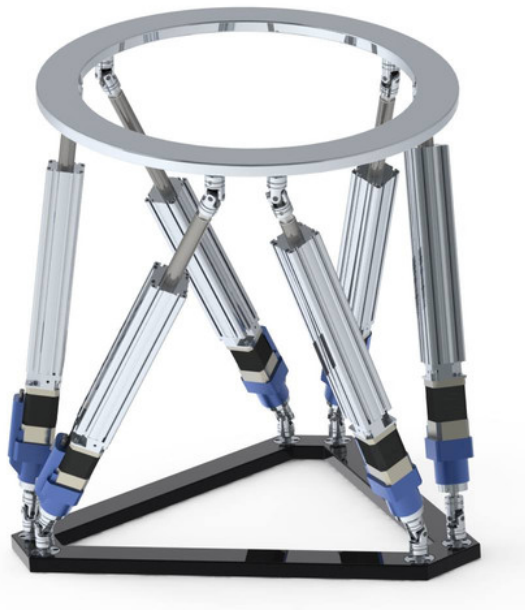
Figure 10: Example of a Stewart platform, reproduced as is from [14]
