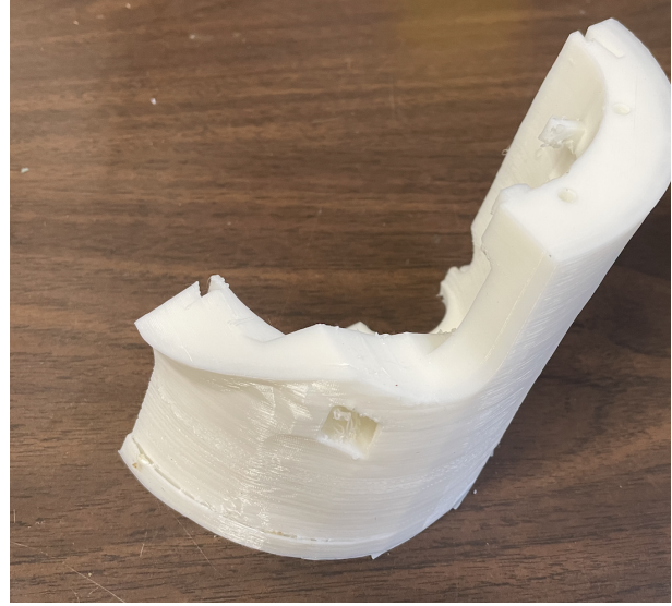
Figure 64: Completed Print of Lattice with Skin in TPU
