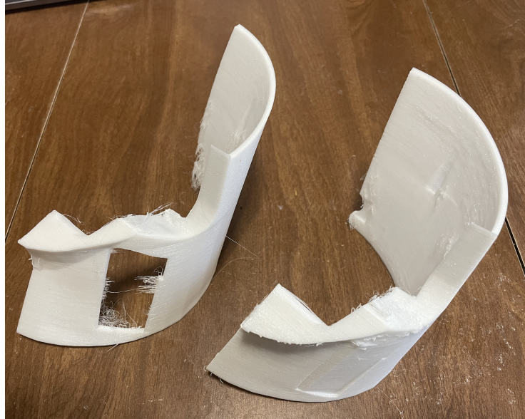
Figure 61: TPU skin test prints (Left 10%, Right 15% infill)
