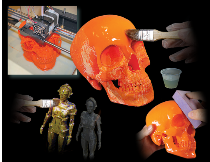
Figure 89: Commercially Available 3D Coating from Smooth-ON, reproduced as is from [35]
