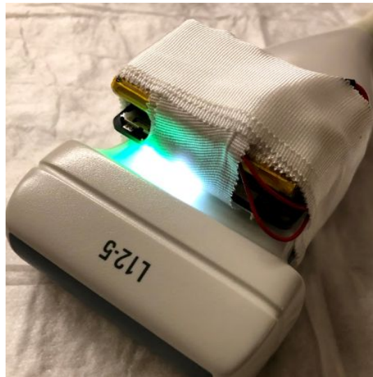
Figure 6.3: Case with Medical Tape on Ultrasound Probe
