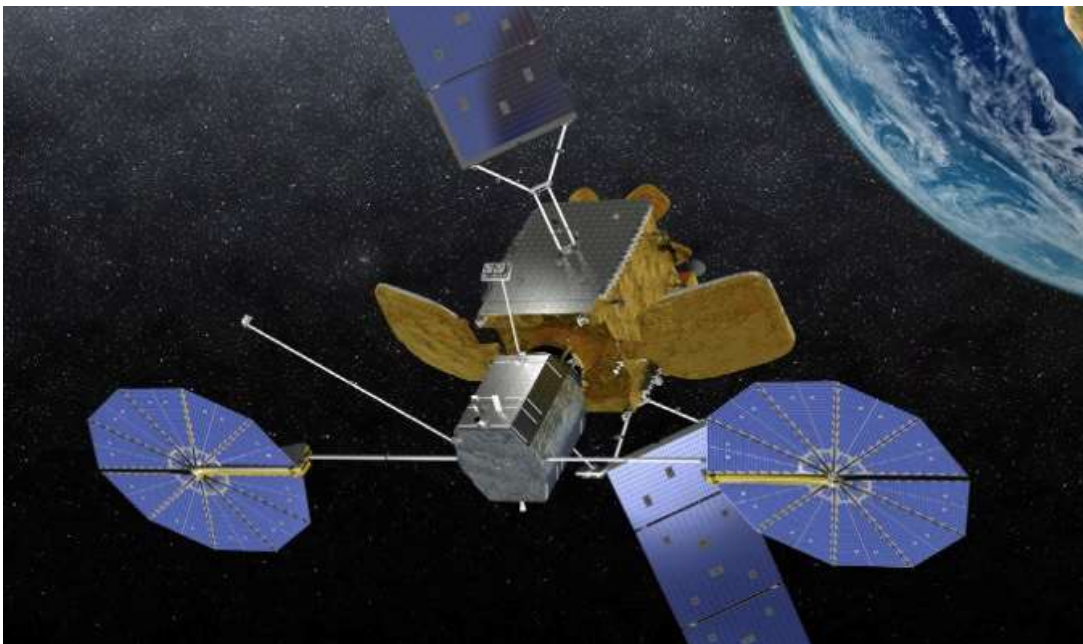
Figure 1: The MEV (foreground) docked with the client vehicle, forming the combined vehicle stack
