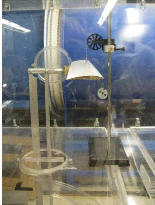
Figure 51: Setup for additional lift calibration data.
