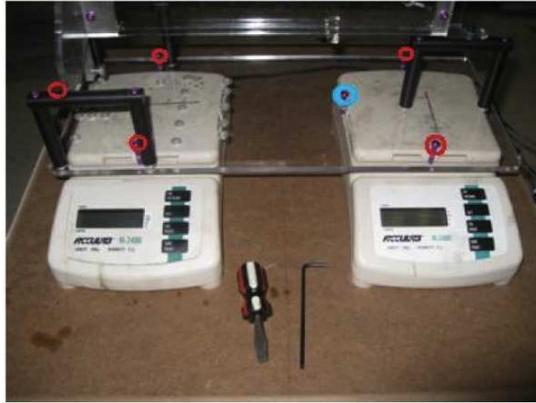
Figure 46: The screws to be backed out are indicated in red and the one to be removed entirely is in blue.
