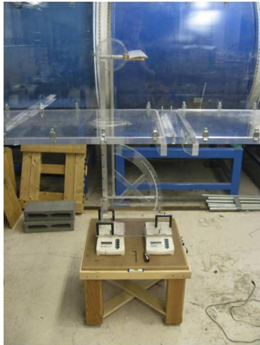
Figure 33: Basic test stand setup for collecting lift data.
