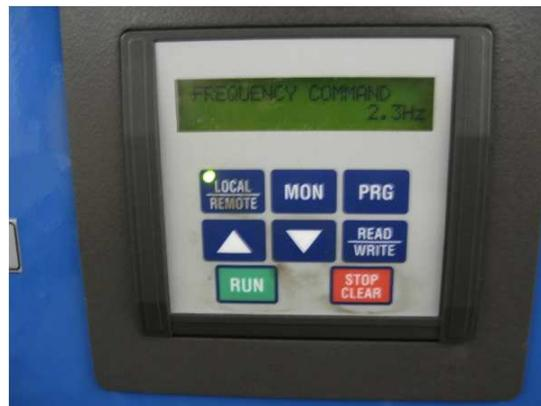
Figure 52: Control panel for setting the wind tunnel speed.
