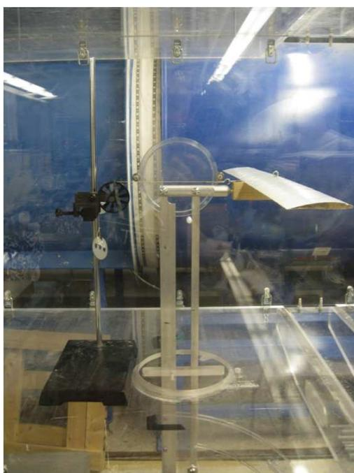
Figure 50: Setup for drag calibration data with a 10g mass.
