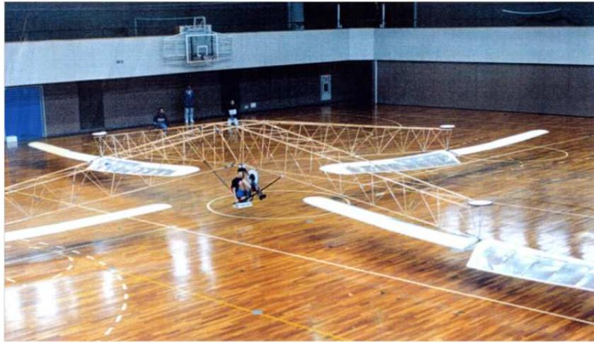
Figure 1: The Da Vinci III human powered helicopter.
