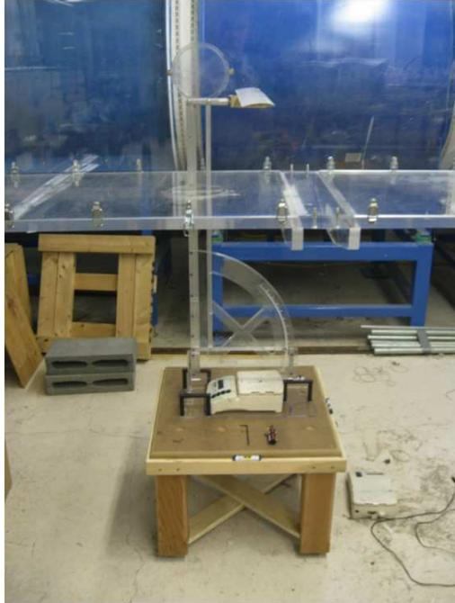
Figure 45: Basic test stand setup for collecting drag data.
