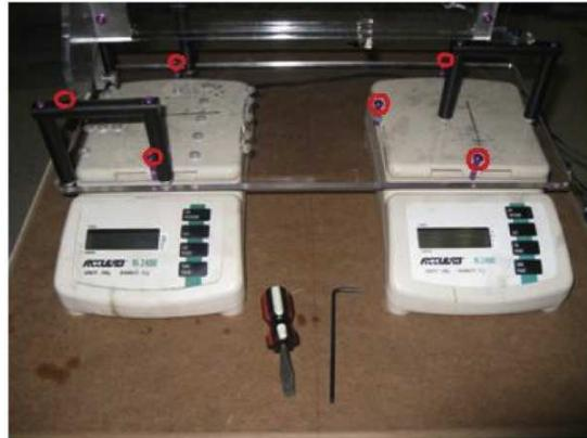
Figure 36: The red circles indicate screw locations to hold the test stand stationary for measuring lift.
