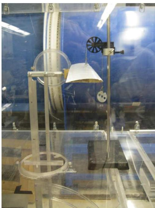
Figure 42: Lift calibration setup with a 10g mass.
