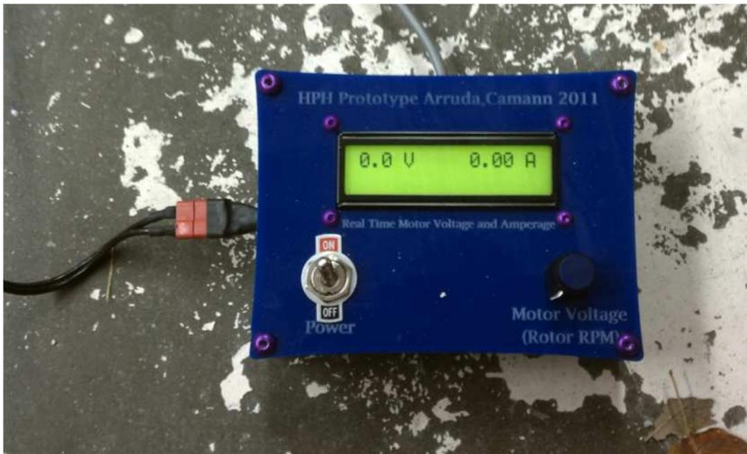
Figure 26: The power supply box with power switch and voltage controller.
