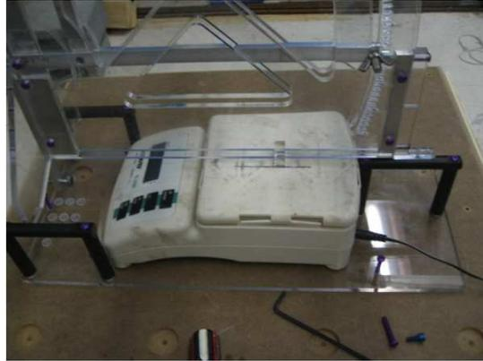
Figure 49: A single scale is place under the test stand.
