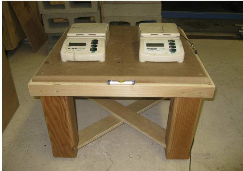
Figure 7: The test table with two scales mounted in the bored holes. The test stand will sit on top of the scales so that lift can be measured.
