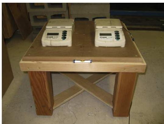
Figure 35: Scales in place for measuring lift.
