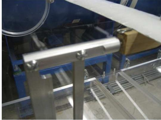
Figure 39: Close-up of the test wing fixed to the stand in the wind tunnel.
