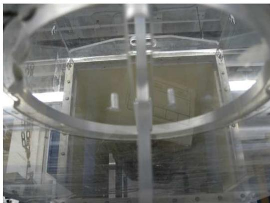
Figure 47: As with lift measurements, make sure the test stand is not in contact with the edges of the access hole.
