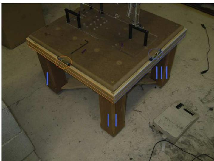
Figure 34: Leveling the test stand table.
