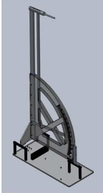
Figure 8: CAD model of the test stand.
