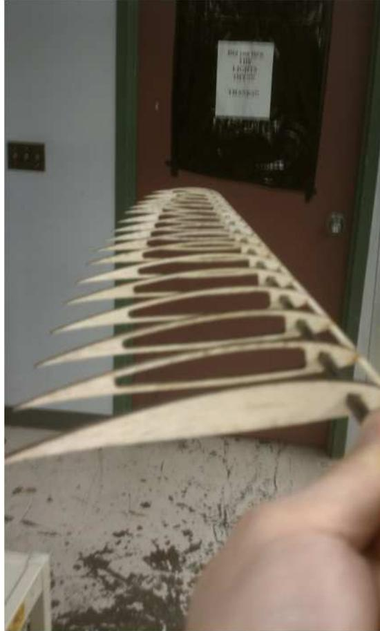
Figure 24: Wing spar with the cut ribs attached. This constitutes one of the four rotor blades.
