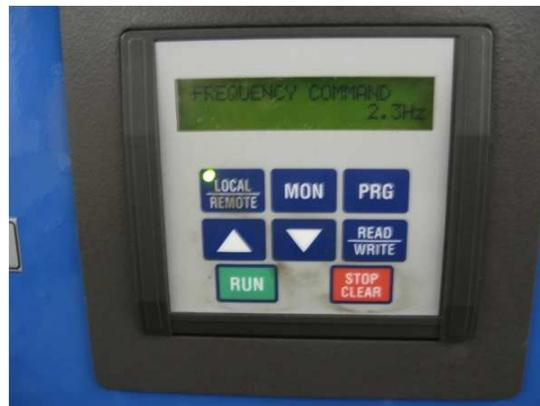
Figure 43: Control panel for setting wind tunnel speed.
