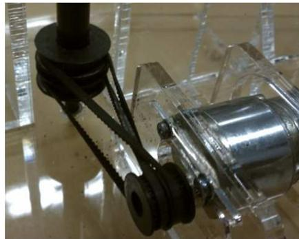
Figure 6: A close-up of the pulleys shows how to produce the counter-rotation.
