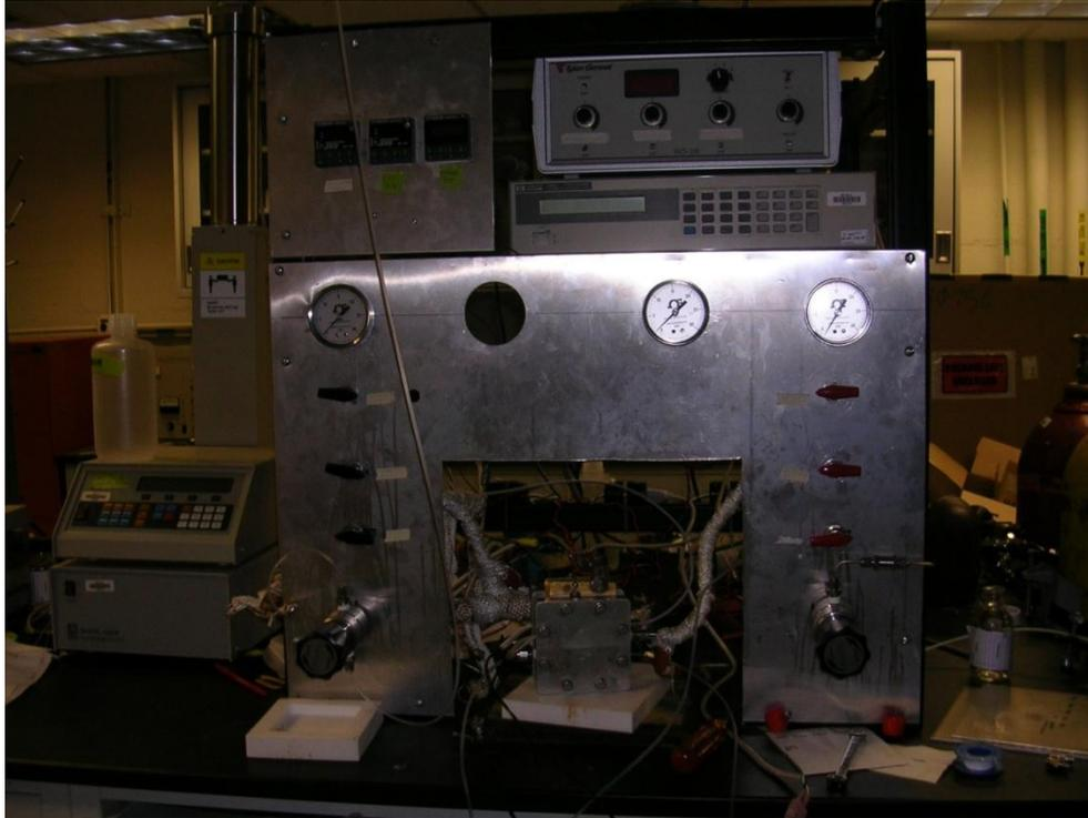
**Figure 28: DMFC Test Station**
