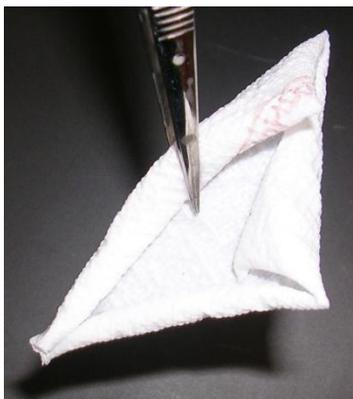
**Figure 30: Photo of a warped carboxylic acid membrane (N982)**
