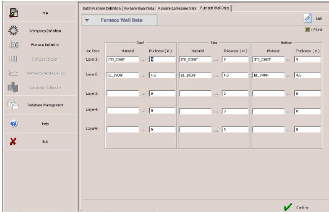
Fig. 3.10 Furnace definition page4 --- furnace wall
