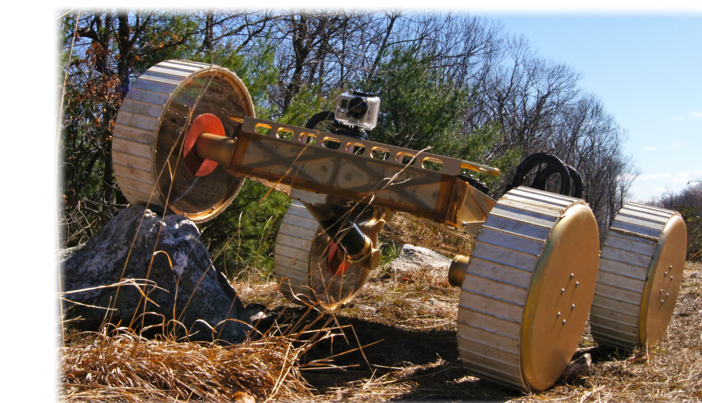
Figure 6 - Overcoming a rock during field testing
