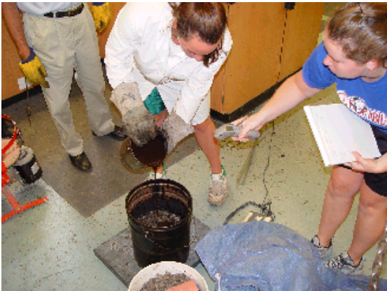
Figure 5. Pouring Emulsion/Asphalt into RAP and Recording Temperatures
