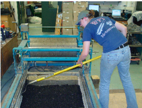
Figure 7. Evenly Spreading the Mix in the Mold
