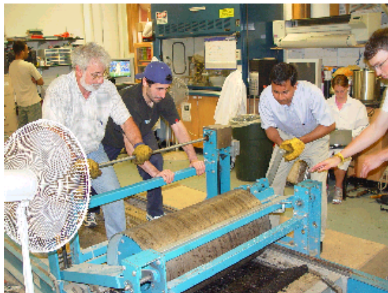
Figure 8. Compacting with Vibratory Roller
