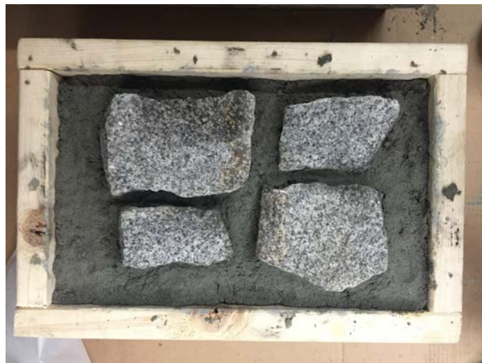
Figure 14: Reinforcement concrete panel with stones and mortar
