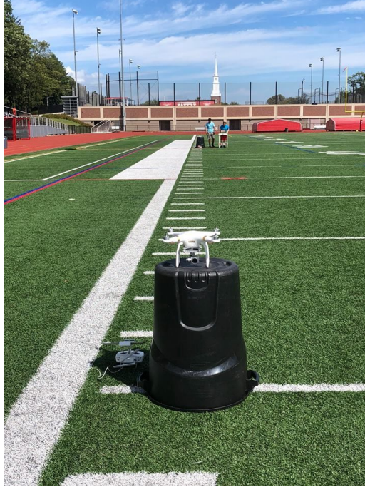
Figure 7: Data Acquisition Test Setup for Path Loss Modeling
