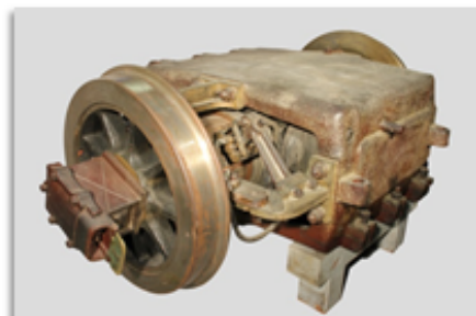
Figure 1: Electric powered motor from a City & South London Railway train. (1996/4695). Manufactured by Crompton 1899/1900
