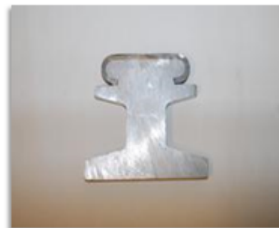
Figure 2: Cross section of an aluminium core railway track (T06). The darker grey part is made out of stainless steel while the rest is aluminium. This rail uses the high conductivity of aluminium to avoid large power losses and the durability of stainless steel to withstand constant wear from the train. When the steel is worn out, it can easily be replaced without removing the entire rail.
