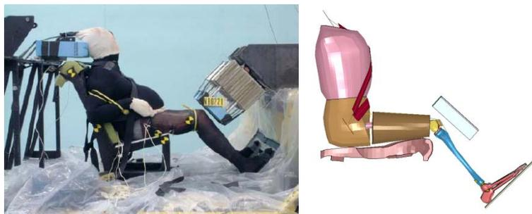
**Figure 21: Initial Sled Test Position in Physical Test (left) and FE Simulation (right)**
