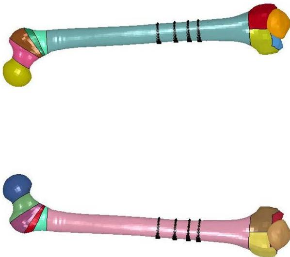
The femur axial forces were measured at the highlighted sections in the above figure. I.D.s 5-8 are on the left leg and start at the knee and move towards the hip. I.D.s 9-12 are on the right leg and move from the hip towards the knee.
