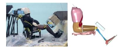
Figure 21: Initial Sled Test Position in Physical Test (left) and FE Simulation (right) Rupp 2002 and Silvestri 2010
