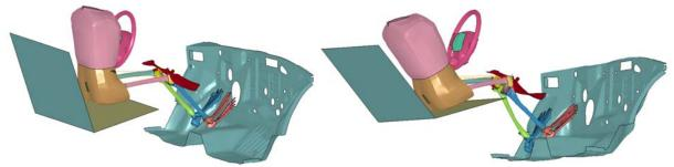
Figure 34: Large Tibia Displacement Relative to the Femur
