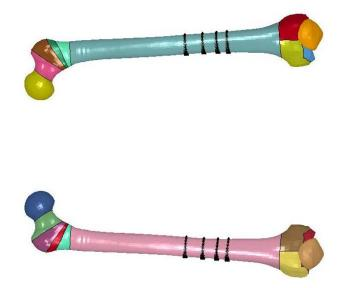
The femur axial forces were measured at the highlighted sections in the above figure. I.D.s 5-8 are on the left leg and start at the knee and move towards the hip. I.D.s 9-12 are on the right leg and move from the hip towards the knee.
